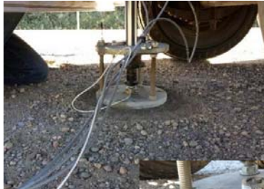
12 in. plate on Gravel
