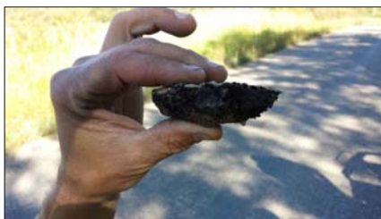
Example of 20 to 30 mm thick chip seal surface.
