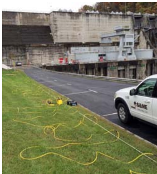
Advanced Geosciences, Inc. (AGI) SuperSting™ R8/IP configured with up to 84 electrodes
