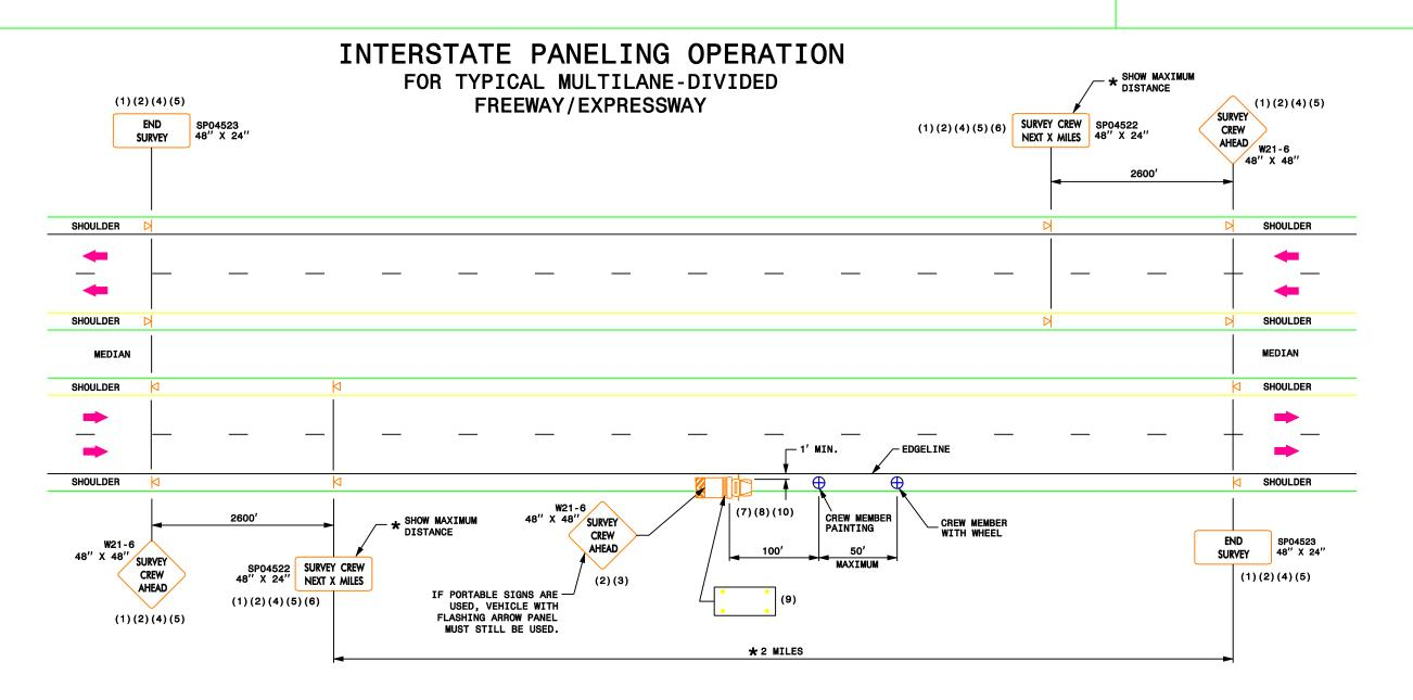
LOCATION: VEHICLE AND/OR CREW MEMBER IS LESS THAN FOUR FEET (4') BUT NO CLOSER THAN ONE FOOT (1') FROM EDGELINE.
