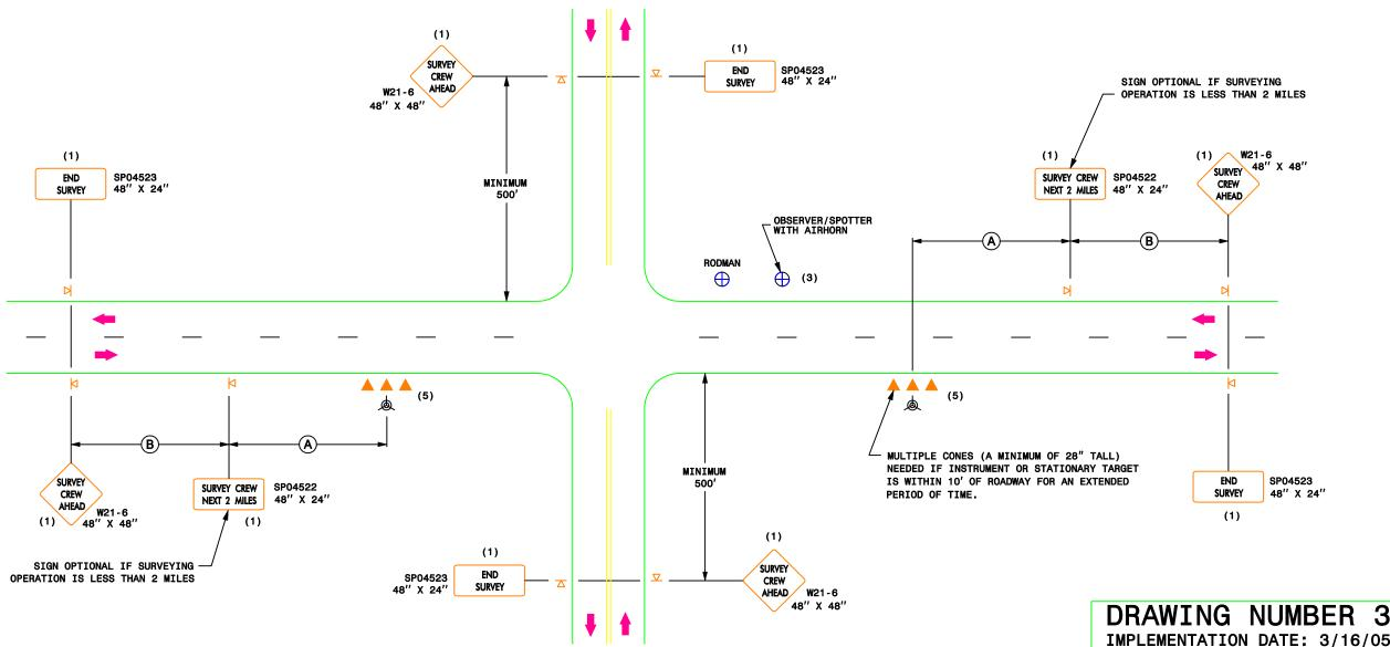
ncdot location & surveys workzone safety signing diagrams.dgn 12/03/2007 09:31:38 AM
