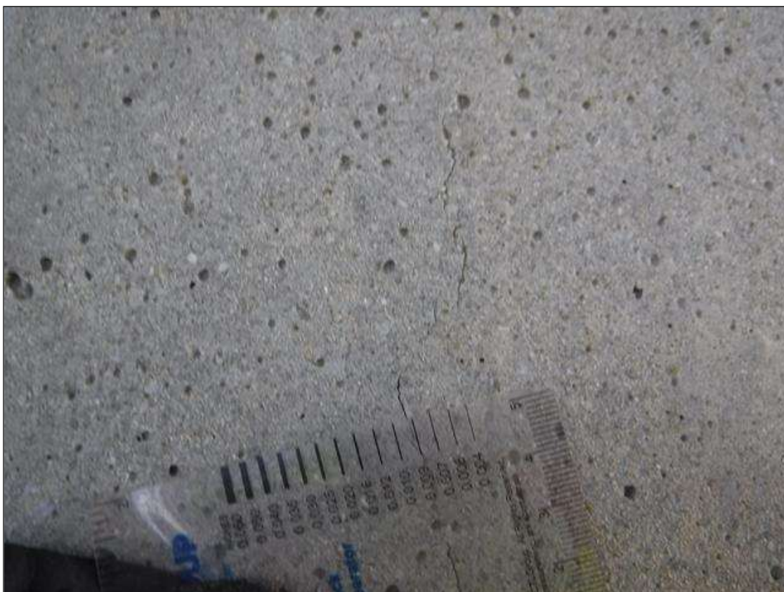
Bent 130 Pile 3: UP TO 3' X 0.009" VERTICAL CRACKS, AT RANDOM THROUGHOUT.
