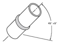
PIPE INCLINATION FIXED (45° ±5°) AND NOT ROTATED DURING WELDING.
