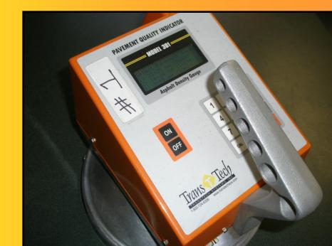
Turn **PQI** on and set testing parameters . . .
