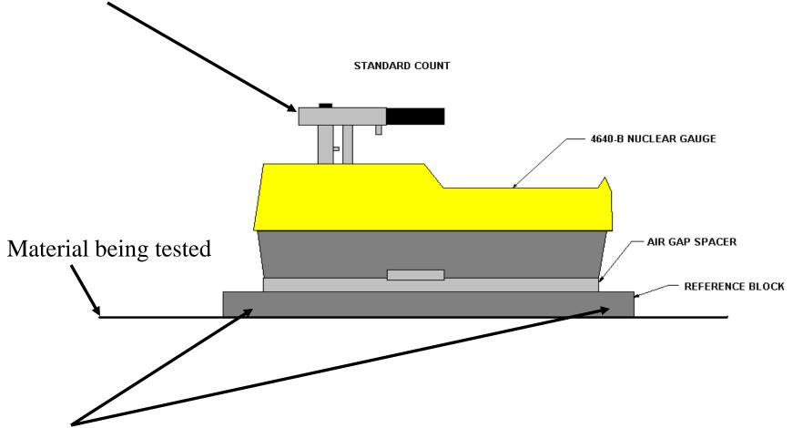
Ensure the surface is dry, flat and the Reference Block does not rock
