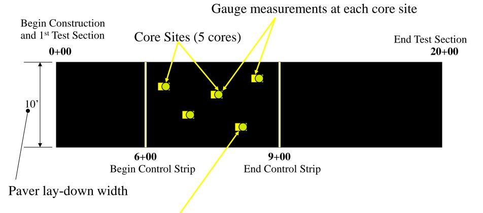
Cores <u>shall not</u> be located until compaction of the Control Strip is completed
