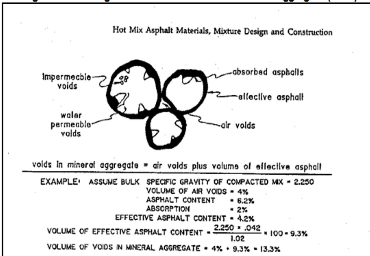
(Note: For simplification the volume of absorbed asphalt is not shown.)
