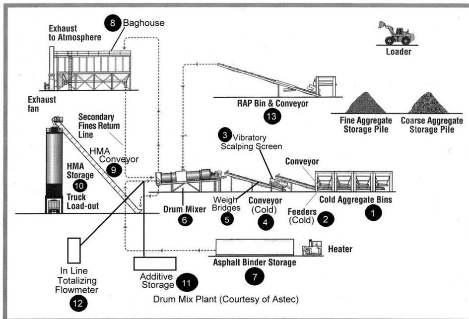
Drum mix plants vary in size and rated capacities from approximately 60 tons per hour up to several hundred tons per hour. A minimum production capacity of 90 tons per hour for drum mix plants is required on all NCDOT construction contracts.
