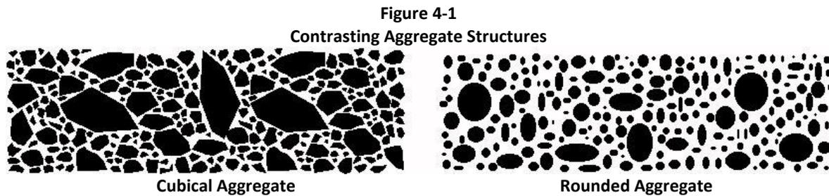
The figure above demonstrates that with more angular (cubical) particle shape and more contact between particles greater resistance to rutting and permanent deformation is achieved. For any given aggregate, the rut resistance increases with the density of the confined particles, which is achieved by dense gradations and adequate compaction. Excessive asphalt in the mix tends to lubricate the aggregate particles and lower the internal friction of the stone framework.
