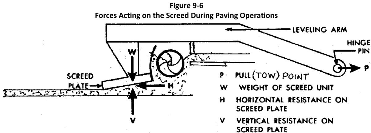
The asphalt mixture must be spread and finished to the required grades, cross sections, thickness and widths shown on the plans and typical sections and to uniform density and texture by the paver. Many working conditions and adjustments can be checked only by the end results or more specifically, by the quality of the mat that is placed. However, before work begins, certain checks on items that would obviously affect the work should be made.
