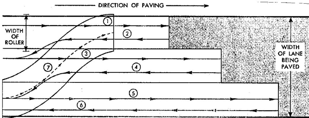
This is a recommended rolling pattern. Every pass of the roller should proceed straight into the compacted mix and return in the same path. After the required passes are completed, the roller should move to the outside of the pavement on cooled material until repeat the procedure.
