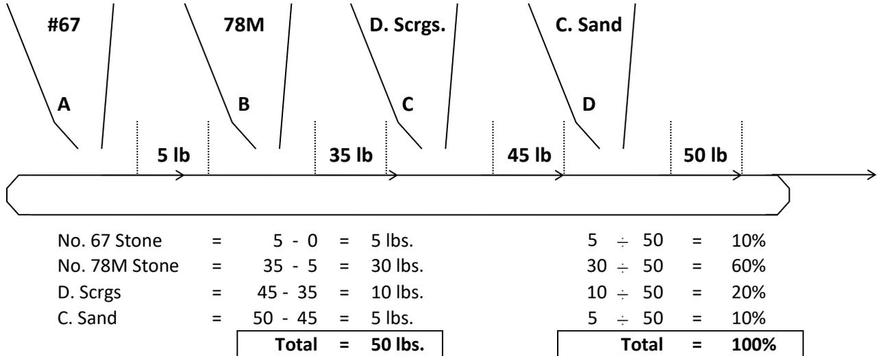
Note: Sample across the entire cross-section of belt for a minimum of two (2) feet.
