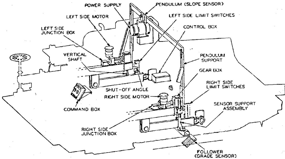
The automatic screed controls should be used all times possible because it can, in most cases, do a much better job than the manual control. If the automatic control equipment malfunctions, the manual controls may be used for remainder of that work day, provided satisfactory laydown is being achieved.
