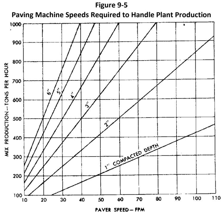
NOTE: Paver speed based on spread 12-ft. wide
