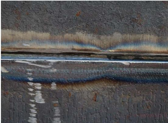
Inadequate back gouge.
