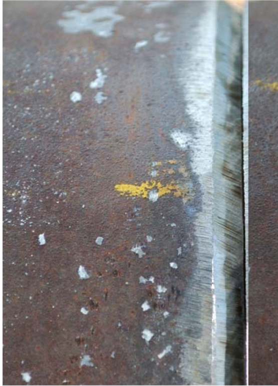
Typical fit-up using a 45 degree Single Bevel.
