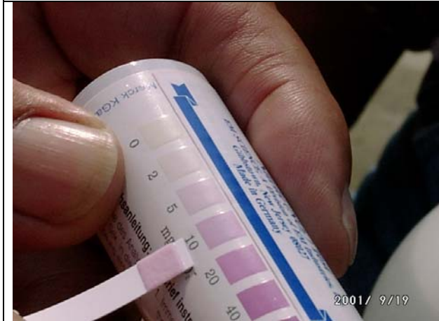
Figure 9: Close up of the scale. This is typical reading of 10 for the first 20 mL dilution.
