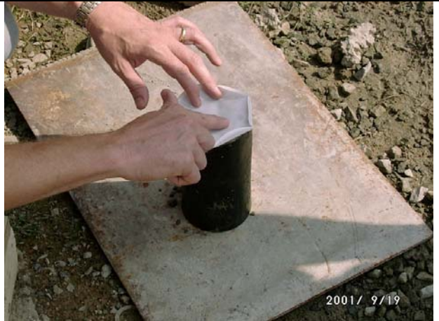
Figure 2: Extracting nitrite-laden bleedwater from the Dead end cylinder in its plastic state.
