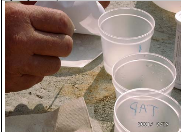
Figure 3: The cups have 20 mL of water in each one. (*TAP water is no longer used. Distilled water ONLY!) The “dot sandwich” is carefully opened and a dot is picked up with a sharp toothpick. TWO per cup.
