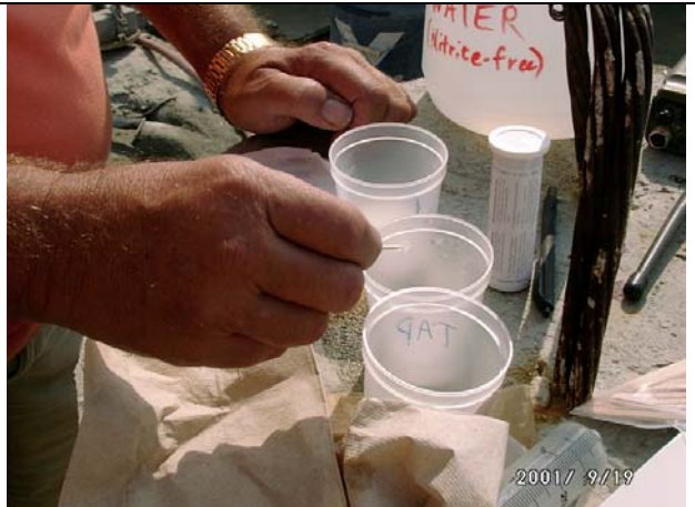
Figure 4: Dots being placed into the second cup. (*TAP water is no longer used. Distilled water ONLY!)
