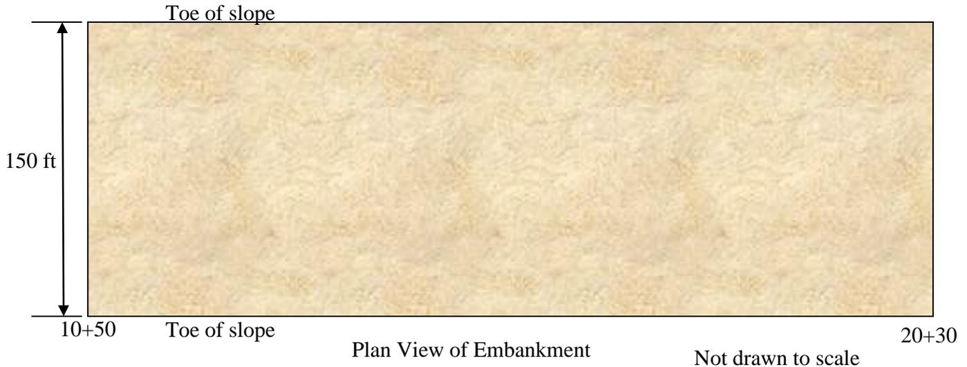
For this example the fill area is 150 feet wide from toe of slope to toe of slope and begins at station 10+50 and ends at station 20+30. The total length of the fill area is 980 feet (2030 – 1050 = 980 feet). Refer to the following steps to randomly determine a test site within the embankment.
