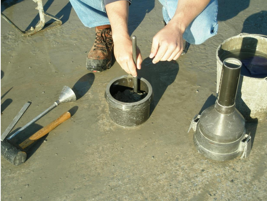
Rod the first layer 25 strokes
