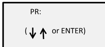
Using the up [↑] or down [↓] arrow keys, scroll through the (flashing) 0-9 digit for the first number to select a value. Once the correct value is displayed press [ENTER].
