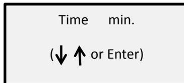
Press the up [↑] or down [↓] arrow keys to scroll through the count time selections. Press [ENTER] to select the desired count time. Once [ENTER] is pressed the gauge will return to “Ready” display.
