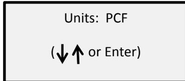
As shown in this example the gauge is set to display readings in pound per cubic foot (PCF). Press [ENTER] to return to the “Ready” display or if metric units are required press the down arrow [↓] for the display:
