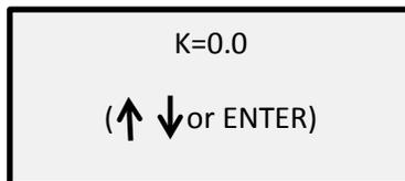
Use the down [↓] and up [↑] arrow keys to enter the calculated  $k$  factor. A negative offset can be entered by pressing the down [↓] arrow **first** and the remaining digits can be keyed in. Once all digits are entered, the device will enable the offset.
