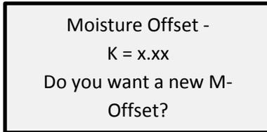
Press [YES] to change the moisture offset (pressing [NO/CE] leaves the factors unchanged).
