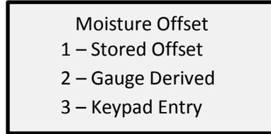
Select [3] and follow gauge prompts to enter the in-place moisture result and nuclear gauge moisture value. The nuclear gauge will calculate the  $k$  factor value. The  $k$  factor value can be saved in memory for future recall if needed.
