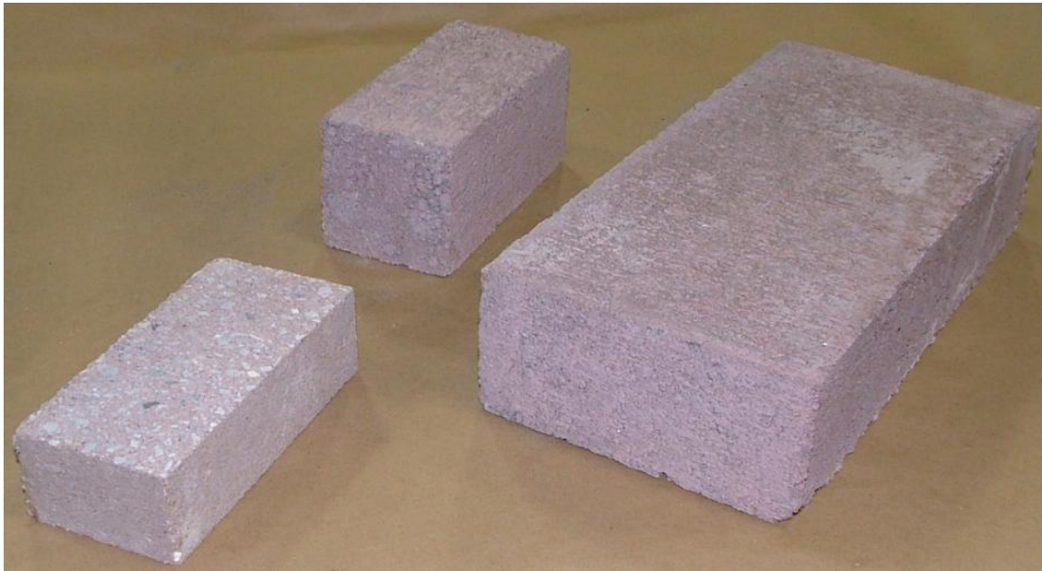
Picture 1. 2"x4"x8", 4"x4"x8", 4"x8"x16" CMUs, all dimensions are nominal (Note: Regular CMU shown is cut from 16" CMU, finish surface shall be the same as the other CMUs)
