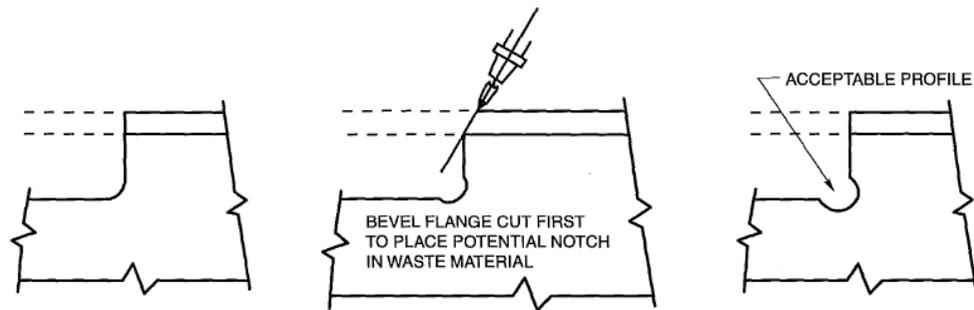
Figure C-3.2—Examples of Good Practice for Cutting Copers
