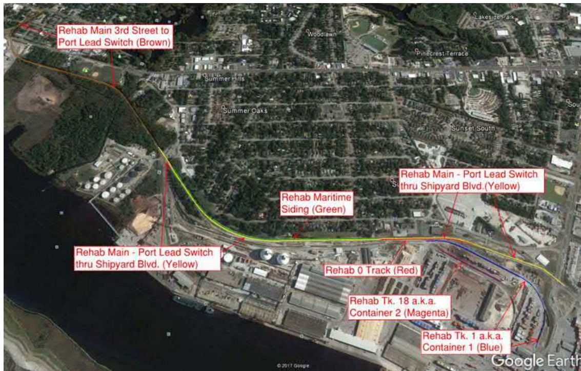
Figure 13: Overview of Improvements Third Street to Port
