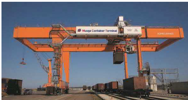
Figure 21: Typical Rail Mounted Gantry Crane
