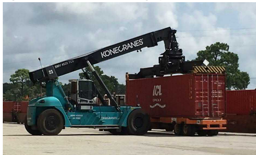
Figure 22: Reach Stacker Loading Operation at the Port
