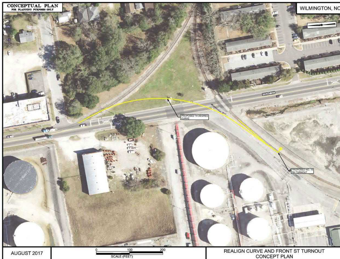
Figure 17: Front Street Improvements
