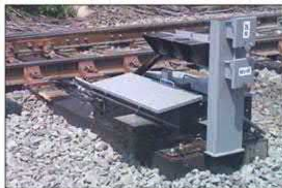
Figure 18: Remote Yard Switch
