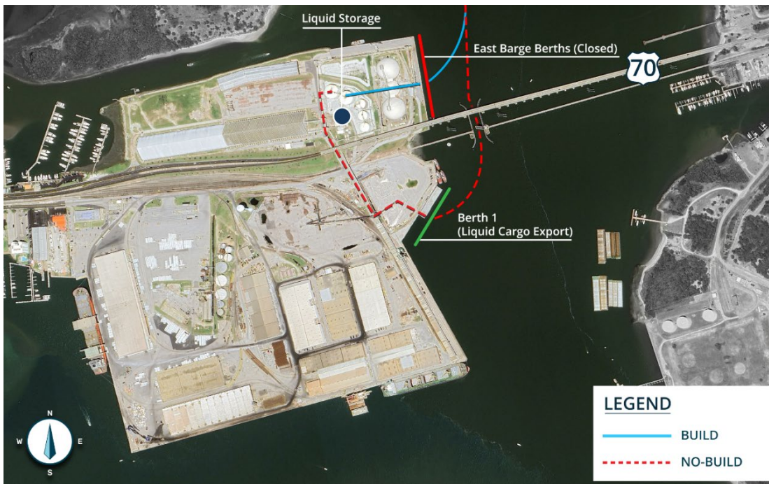
Figure 3. Without the Project, liquid barges are required to navigate beneath the Newport River (US 70) Bridge to Berth 1, where cargo is pumped 1,400' (280%) farther using rented equipment that is less efficient with more safety risks.
