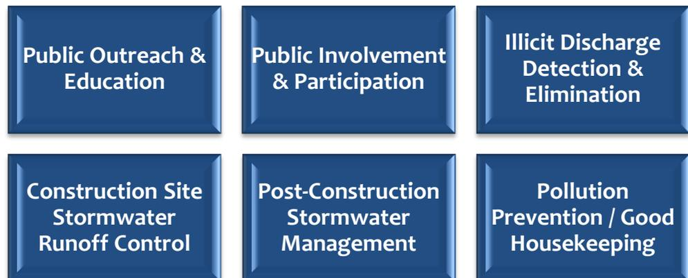
Figure 1.2 NPDES minimum control measures
