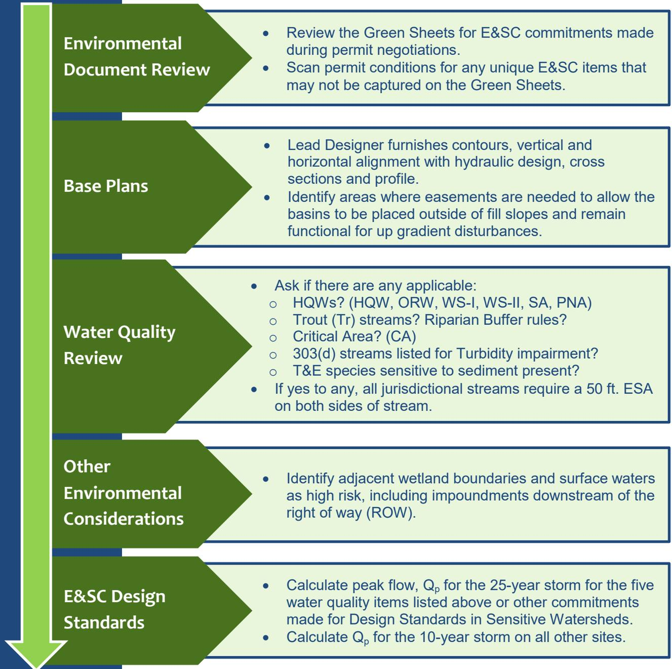
Figure 3.1 Steps to follow before developing the E&SC plans.
