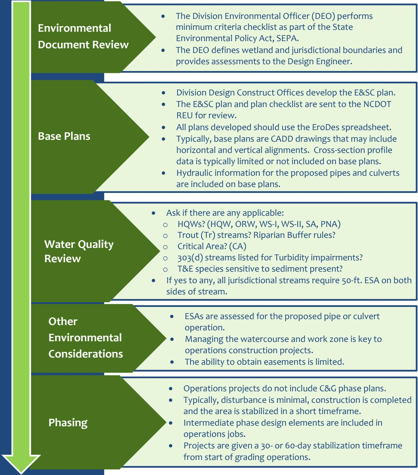
**Figure 3.9 Steps to follow before developing the E&SC plans.**
