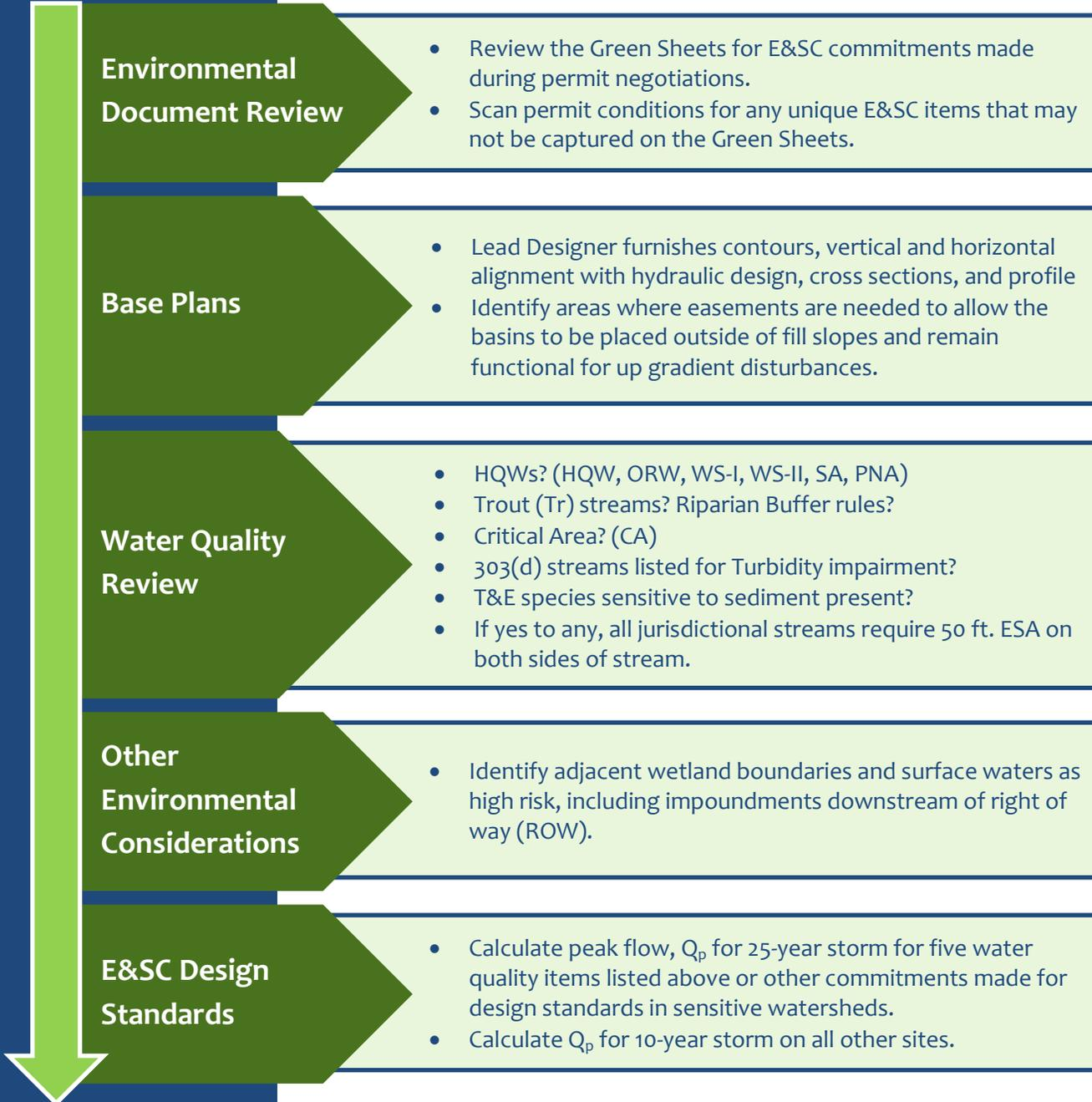
Figure 3.7 Steps to follow before developing the E&SC plans.
