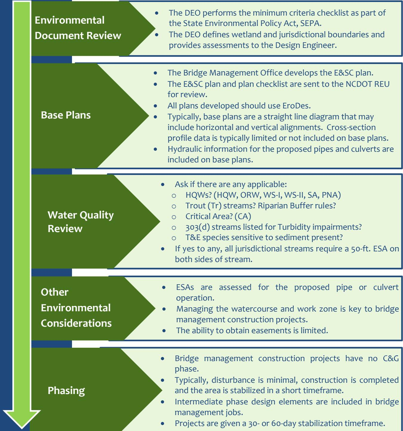
Figure 3.11 Steps to follow before developing the E&SC plans.
