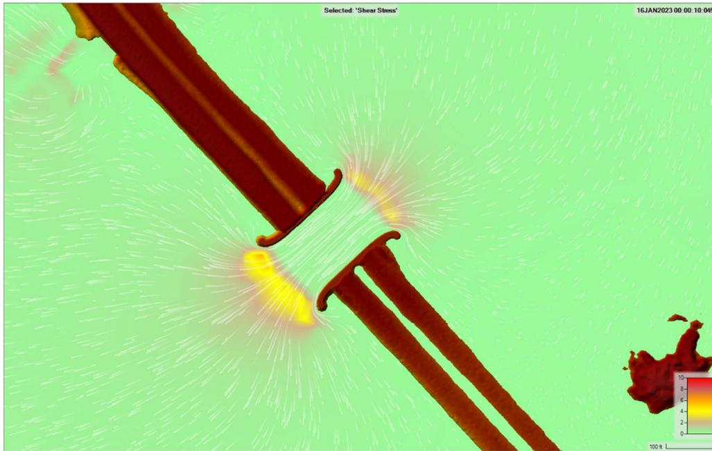
Figure 4.2I. Bridge #4 Shear Stress (100-Yr), Guide Banks
