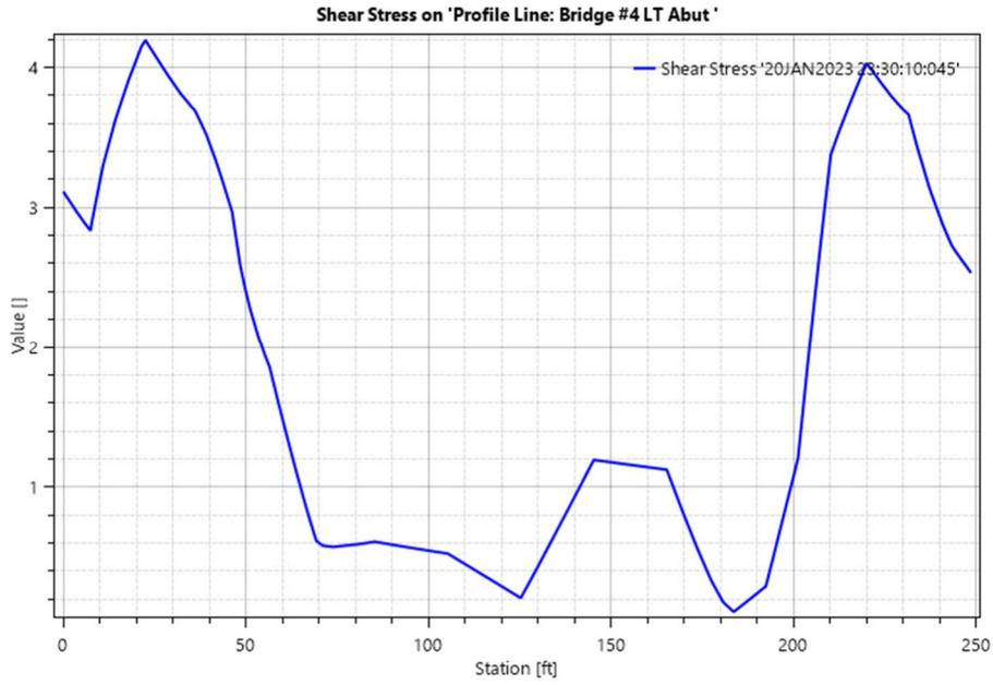
Figure 4.2N. Bridge #4 Left Abutment Shear Stress (500-Yr), Existing Conditions
