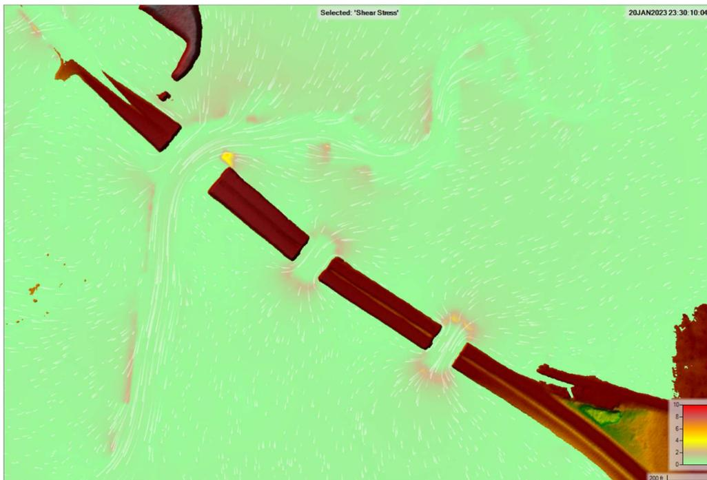
Figure 3.1.2.2D Bridges #1-3 500-Year Shear Stress
