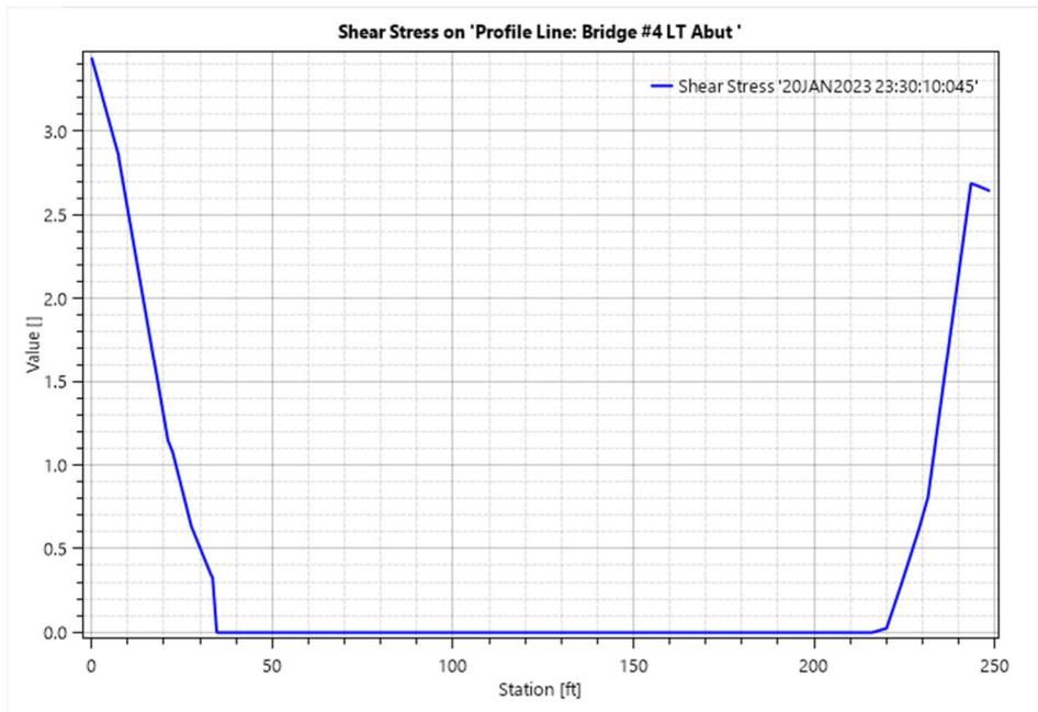
Figure 4.2O. Bridge #4 Left Abutment Shear Stress (500-Yr), Guide Banks
