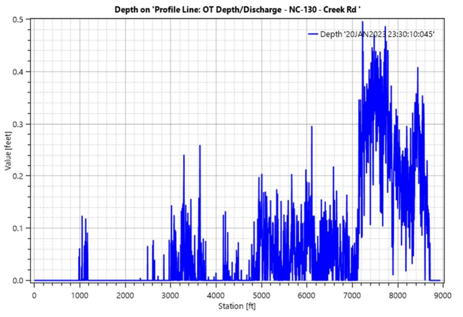
Figure 3.1.2.1P. 500-Year Overtopping Depth, EB Lanes (NC-130 to Creek Rd.)
