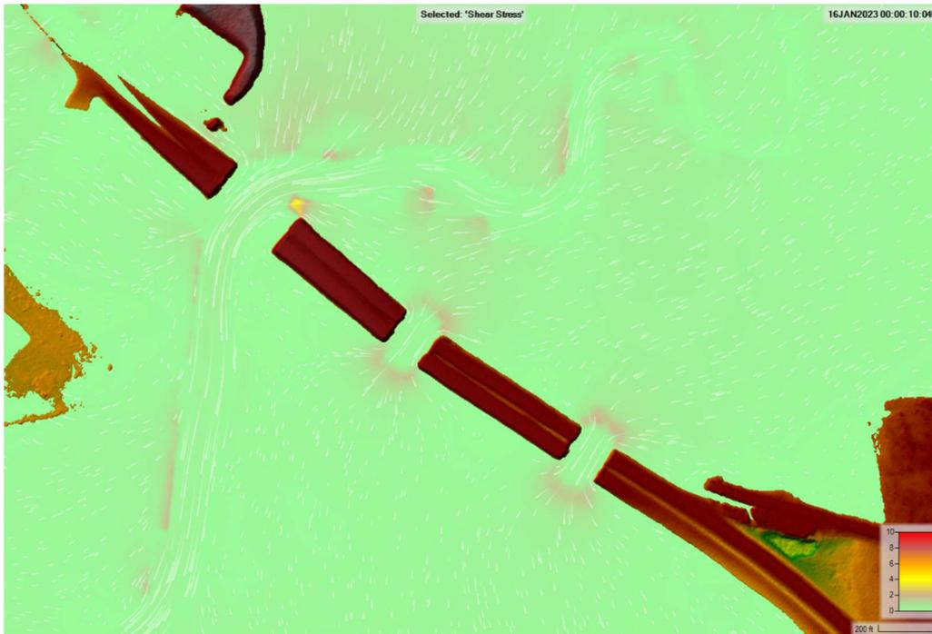
Figure 3.1.2.2C Bridges #1-3 100-Year Shear Stress
