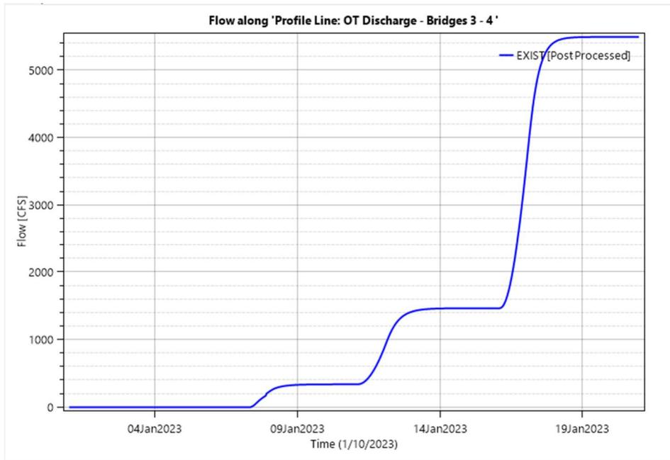
Figure 4.3H. Overtopping Flow Between Bridges #3 & #4 (Existing)
