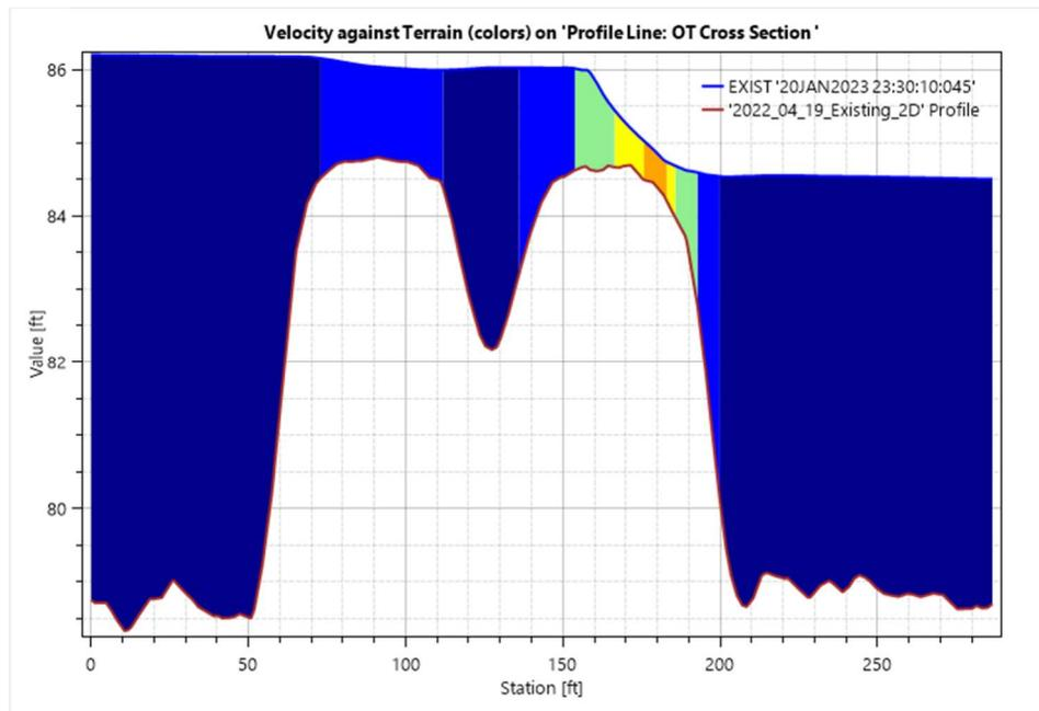
Figure 3.1.2.1K. 500-Year Water Surface & Terrain Example Across Overtopping Location
