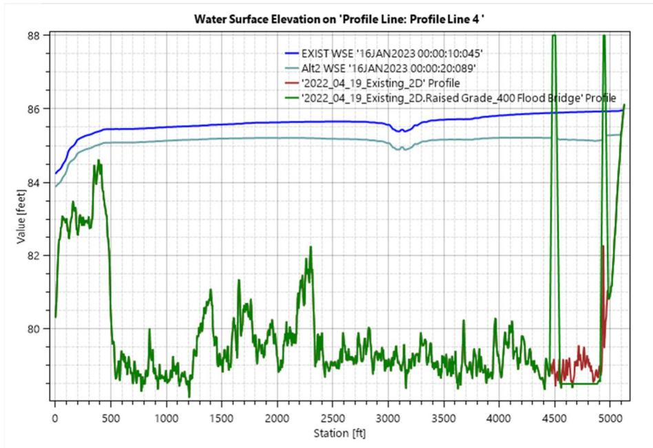
Figure 4.3F. 100-Yr Water Surface Elevation Comparison Along Upstream Embankment
