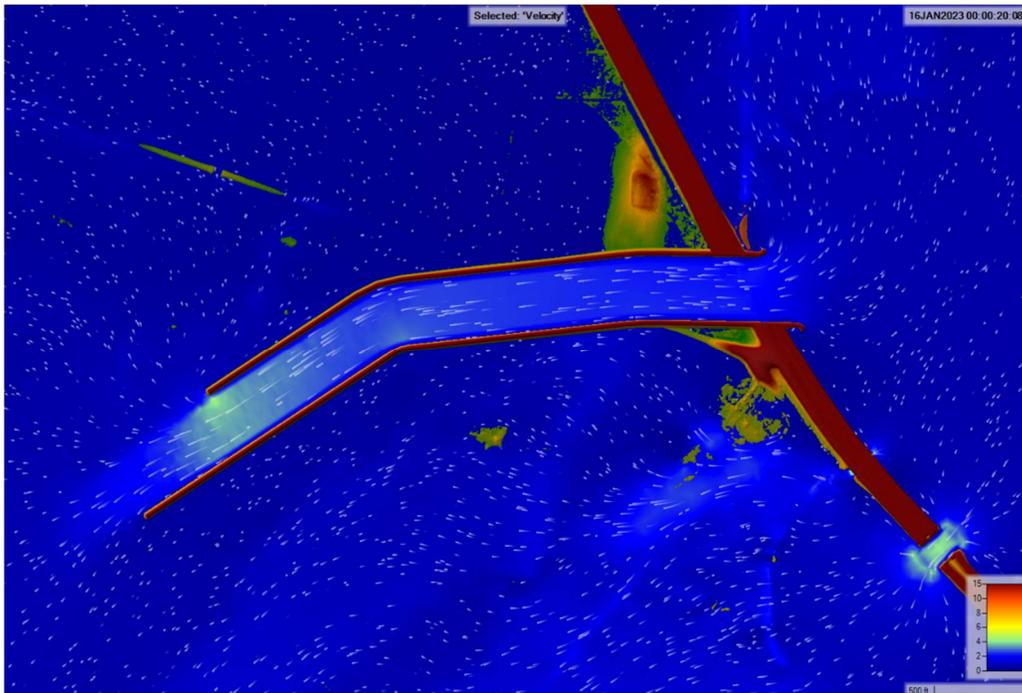
Figure 4.3C. 100-yr Velocities and Flow Patterns for Proposed Floodplain Bridge and Channel
