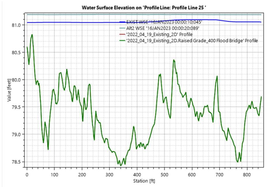
Figure 4.3M. 100-Yr Water Surface Elevation Comparison at 20296 NC-130
