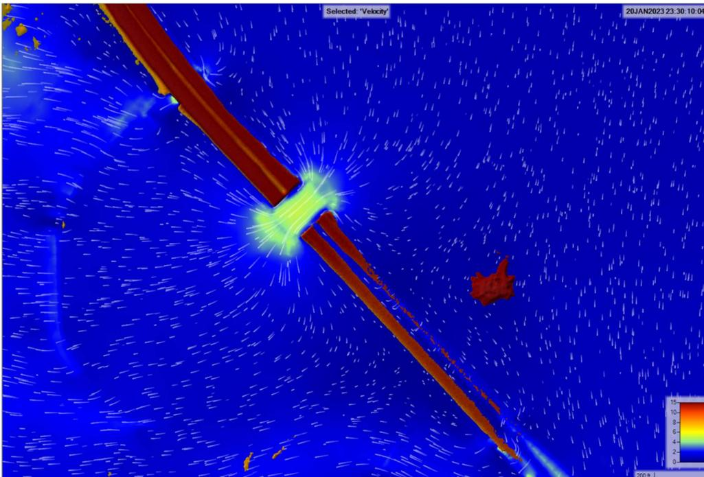
Figure 3.1.2.2F Bridge #4 & Culvert #4 500-Year Velocity
