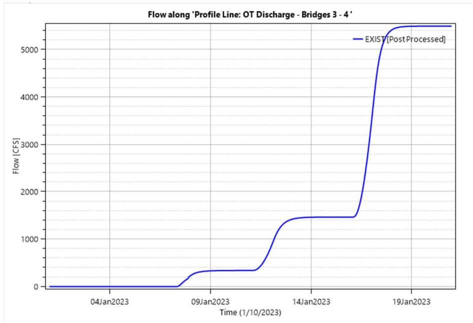
Figure 3.1.2.1S. Overtopping Flow Across EB Lanes (Bridge #3 to Bridge #4)
