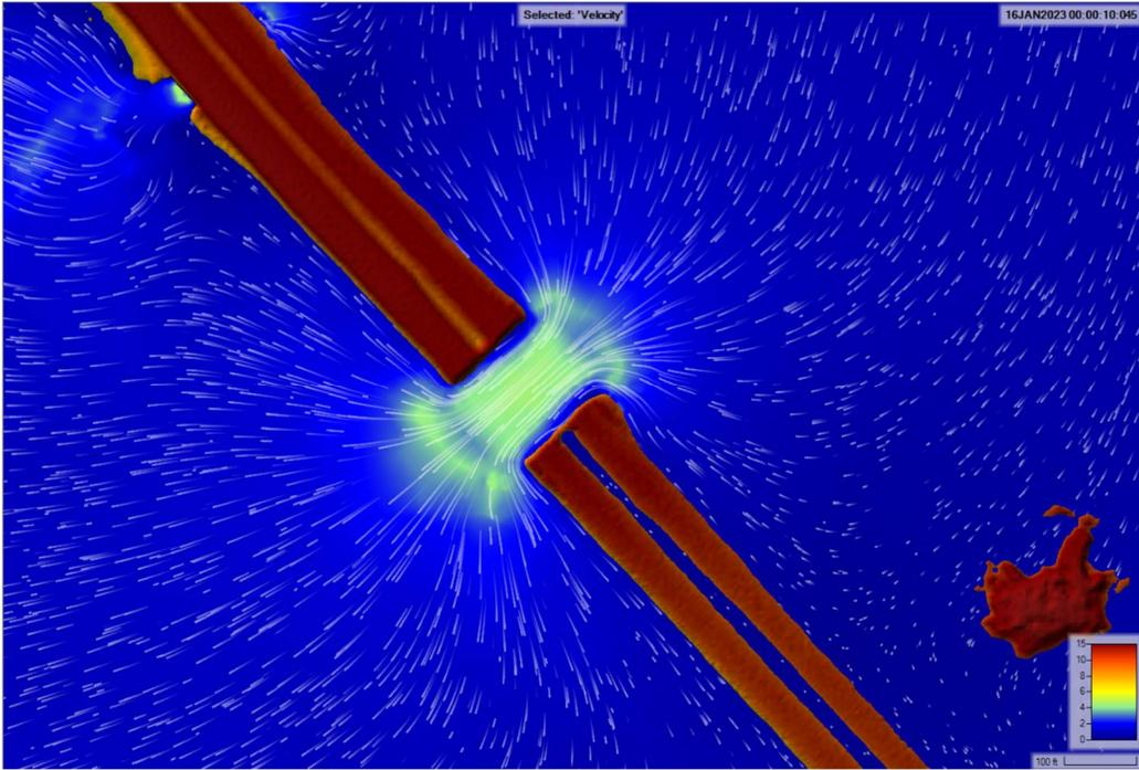
Figure 4.2F. Bridge #4 Velocities and Flow Patterns (100-Yr), Existing Conditions
