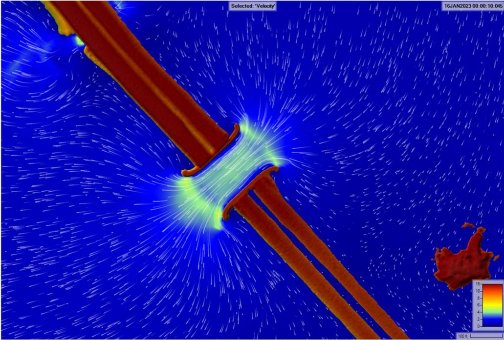
Figure 4.2G. Bridge #4 Velocities and Flow Patterns (100-Yr), Guide Banks
