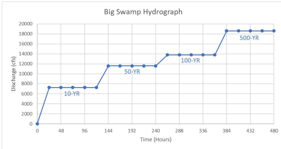
Figure 3.1.1B. Stepped Flow Hydrograph Upstream Boundary Condition on Big Swamp
