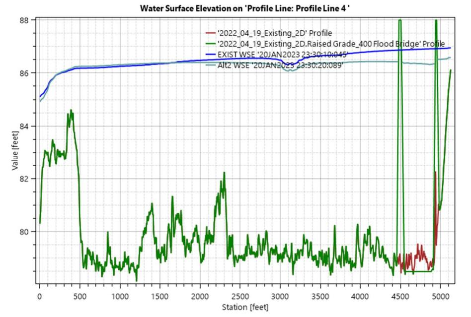
Figure 4.3G. 500-Yr Water Surface Elevation Comparison Along Upstream Embankment
