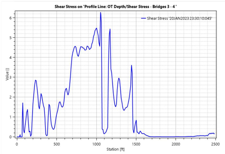
Figure 3.1.2.1L. 500-Year Overtopping Shear Stress, Shoulder of EB Lanes (Bridge #3 to Bridge #4)
