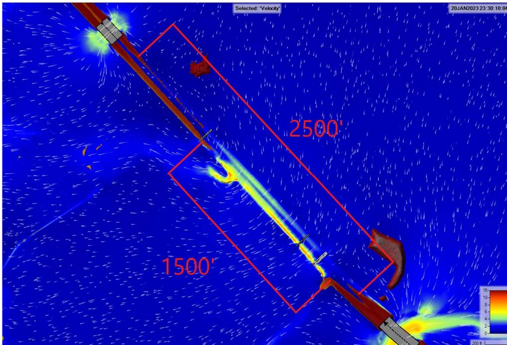
Figure 3.1.2.1I. 500-Year Overtopping & Velocities (Bridge #3 to Bridge #4)
