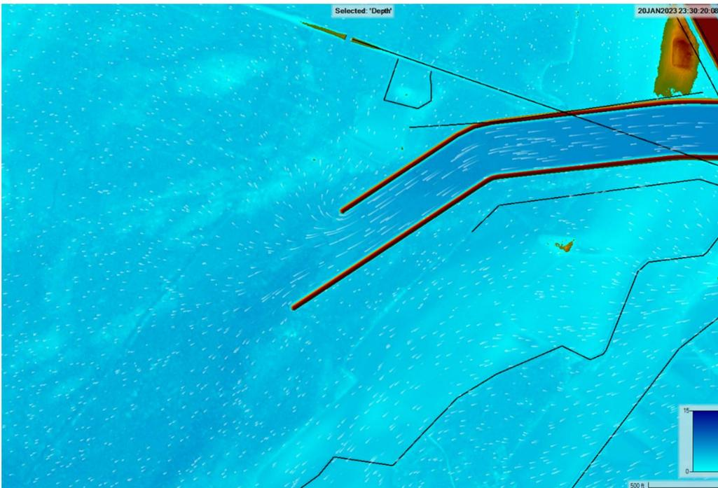
Figure 4.3L. 500-Yr Depth and Flow Patterns at 20296 NC-130 with Flood Channel
