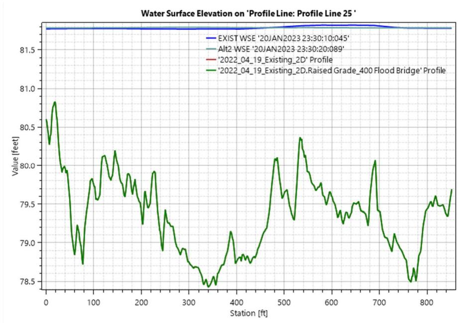
Figure 4.3N. 500-Yr Water Surface Elevation Comparison at 20296 NC-130
