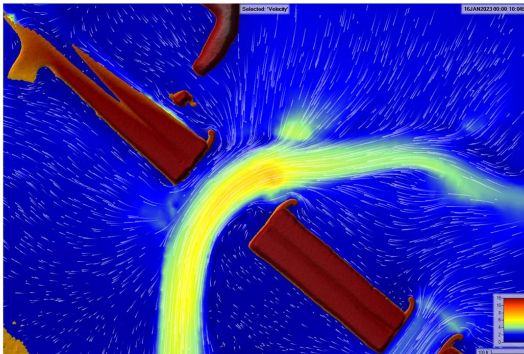
Figure 4.2C. Bridge #3 Velocities and Flow Patterns (100-Yr) with Guide Banks
