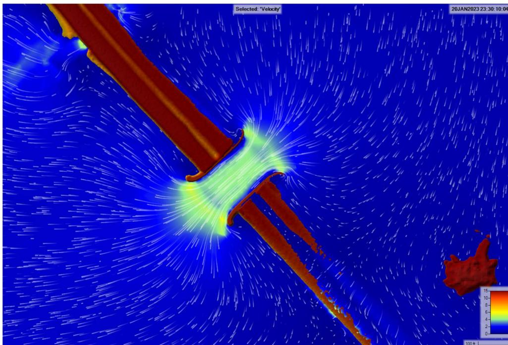
Figure 4.2K. Bridge #4 Velocities and Flow Patterns (500-Yr), Guide Banks
