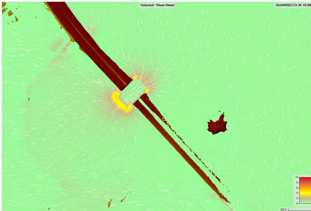
Figure 3.1.2.2H Bridge #4 & Culvert #4 500-Year Shear Stress
