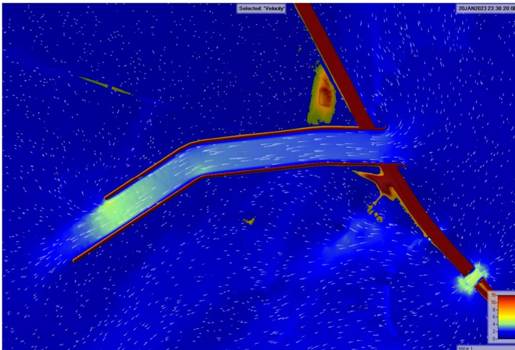
Figure 4.3D. 500-yr Velocities and Flow Patterns for Proposed Floodplain Bridge and Channel
