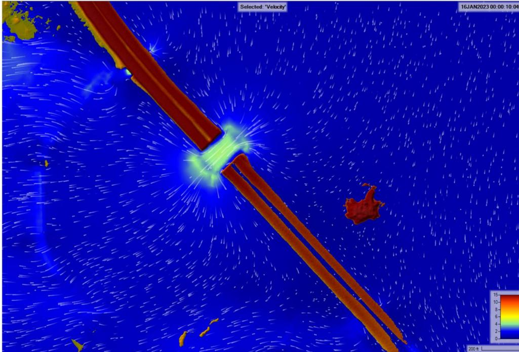
Figure 3.1.2.2E Bridge #4 & Culvert #4 100-Year Velocity
