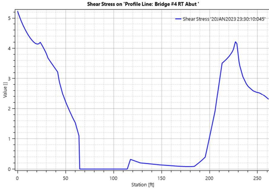
Figure 4.2P. Bridge #4 Right Abutment Shear Stress (500-Yr), Existing Conditions
