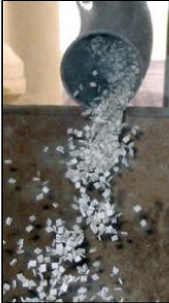
Ultrafiber 500 ® cellulose fibers being added into a concrete mix – image from Ultrafiber 500 ® brochure
