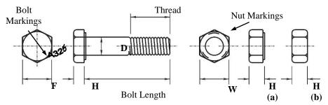
Figure 1072-1. Bolt and nut description. Bolt and nut marking varies. Refer to Subarticle 1072-5(B). F is the width across the flats of the bolt. H is the height of the bolt or nut. Nuts may be washer facing as in (a) or double chamfered as in (b). D is the bolt diameter and nominal bolt size. W is the width across the flats of the nut.
