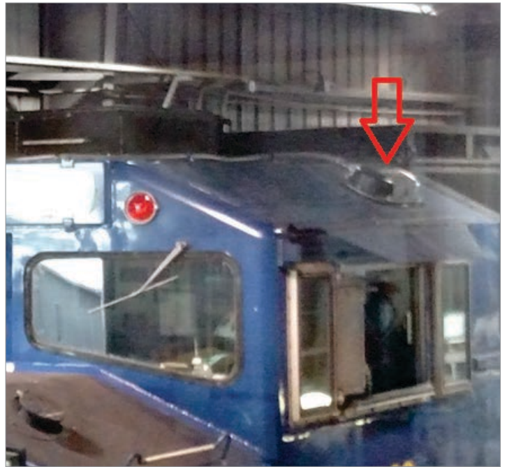
A Wi-Fi antenna is mounted on top of a locomotive cab to send and receive communications.
