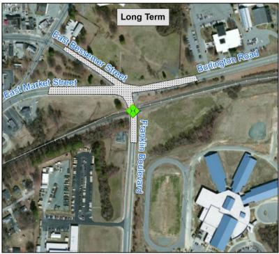
Long Term: Grade-separate Franklin Boulevard by tunneling the street under the tracks, creating a railroad bridge overpass. Creating an underpass also requires that the intersecting streets north of the tracks be regraded lower to meet the new lower elevation of Franklin Boulevard.
