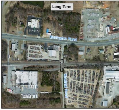
Long Term: Full-closure of Maxfield Road crossing (inset, center left), contingent on Naco Road east-west extension between grade-separtion/street realignment of Ward Road (inset, west) and Wagoner Bend Road (inset, right). Full-closure of Buchanan Church Road (inset, center right) is also proposed.
