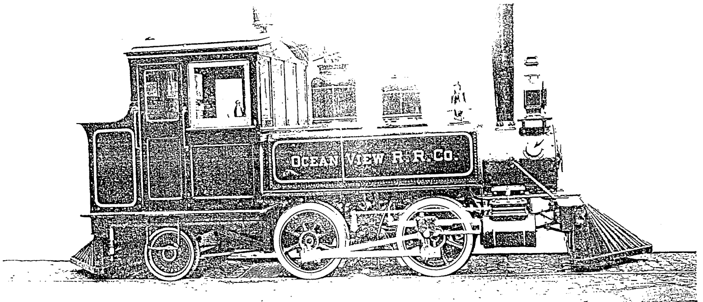
3) This class 0-4-2 tank engine was built by the Baldwin Locomotive Works for the Ocean View Railroad of Wrightsville Beach in 1889. She was brought to Wilmington on May 8, from Philadelphia, and put into service May 21.
