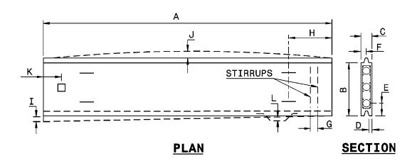
TABLE 1078-6 TOLERANCES FOR PRESTRESSED SHEET PILES
