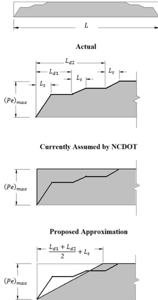
**Figure 5-1** Approximation of the moment profile due to prestressing as affected by debonding and transfer length.
