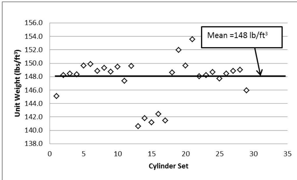
**Figure 5-2** Measured unit weight of concrete cylinders.
