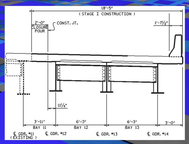
Number of Girders = 3 Skew Angle = 102 degrees Girder Length = 106 ft Interior girder load = 0.801 k/ft Left Ext. girder load = 0.657 k/ft Right Ext. girder load = 0.804 k/ft
