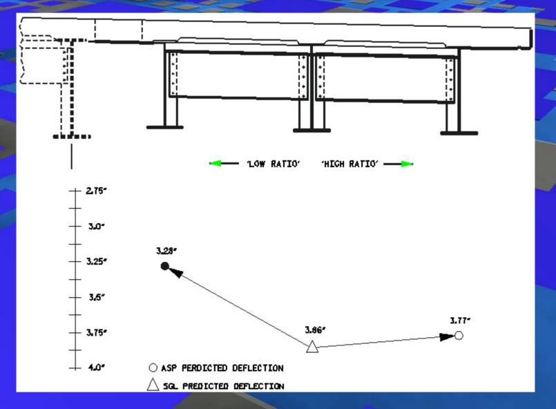
Simple Span - Unequal Exterior-to-Interior Girder Load Ratios
