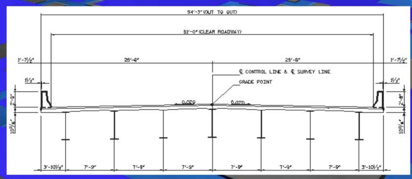
Number of Girders = 7 Skew Angle = 46 degrees Girder Length = 123.83 ft Interior girder load = 2.0 k/ft Left Ext. girder load = 1.7 k/ft Right Ext. girder load = 1.7 k/ft
