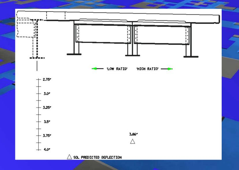
Simple Span - Unequal Exterior-to-Interior Girder Load Ratios
