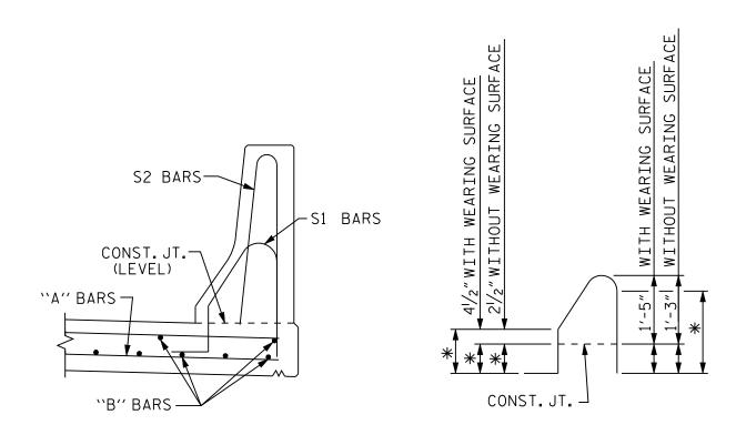
DETAIL FOR COMPUTING LENGTH OF S1 BAR
