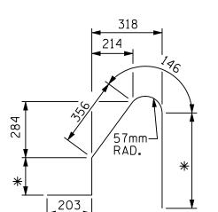
THE LENGTH OF THE VERTICAL LEGS OF THE S1 BARS SHOULD BE COMPUTED IN SUCH A MANNER THAT THE S1 BARS WILL REMAIN PERPENDICULAR TO THE CONSTRUCTION JOINT WITH THE TOTAL LENGTH OF THE S1 BAR DETAILED TO THE NEAREST 20mm. IF THERE IS A SMALL VARIATION IN THE LENGTH OF THE VERTICAL LEGS OF THE S1 BAR, THE SAME BAR MAY BE USED ON BOTH SIDES OF THE BRIDGE.
