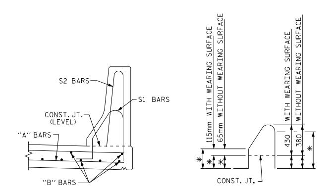
DETAIL FOR COMPUTING LENGTH OF S1 BAR
