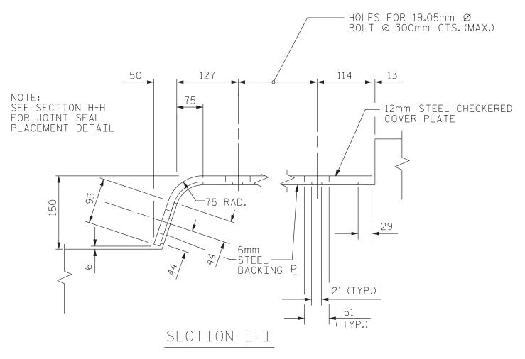
SIDEWALK WITH FOAM JOINT SEAL
