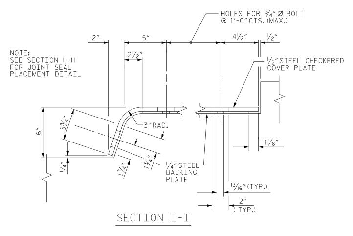
SIDEWALK WITH FOAM JOINT SEAL
