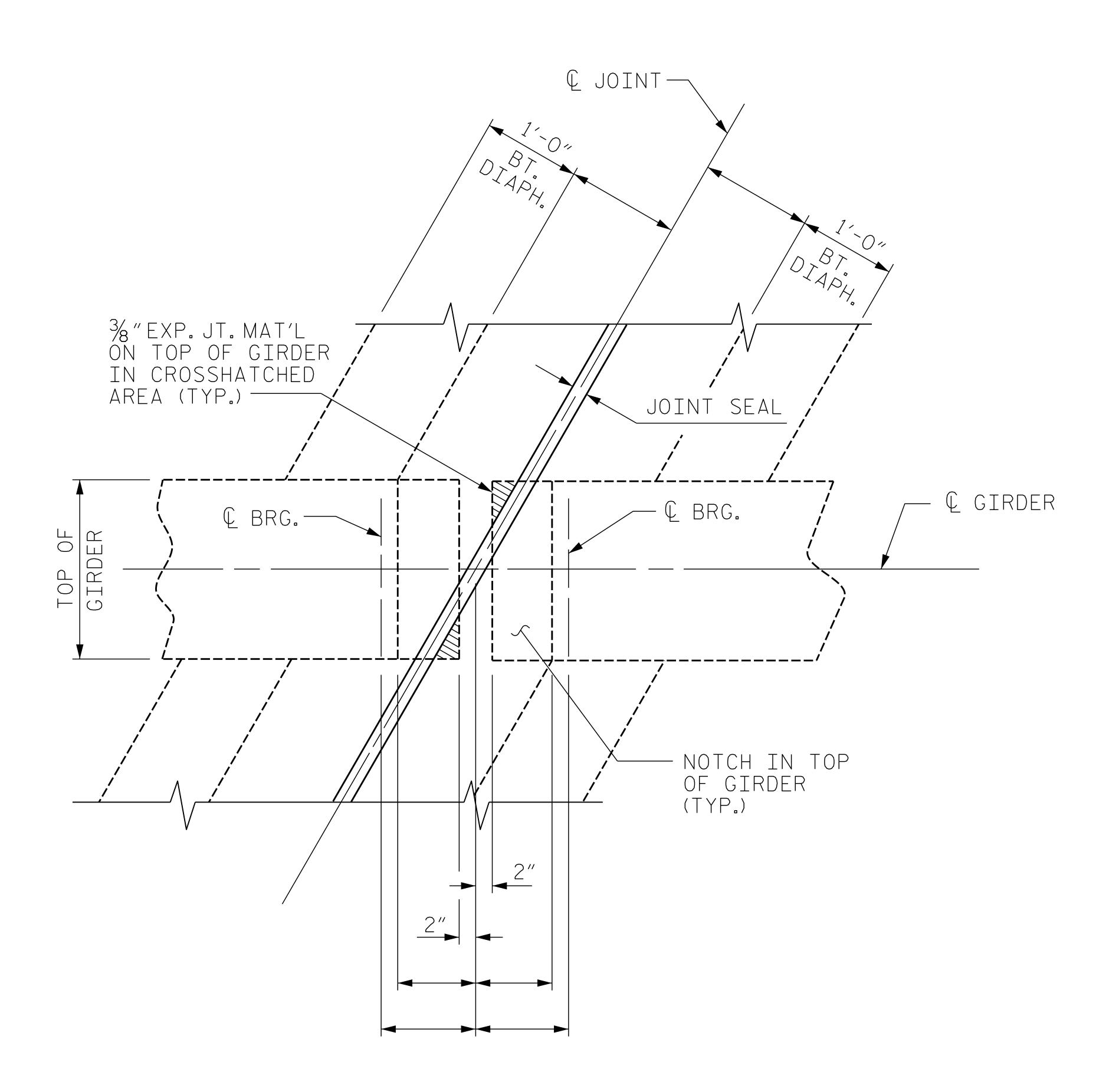
PLAN OF GIRDER END @ BENT
