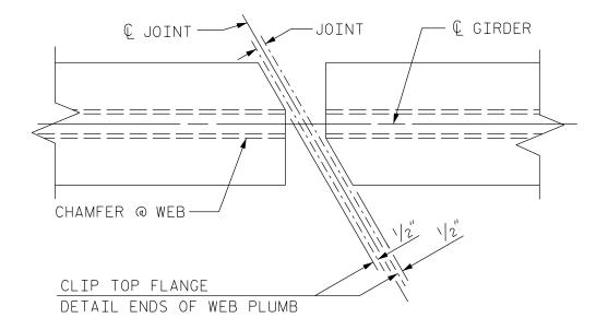
TOP FLANGE AT EXPANSION JOINT NOTE: DO NOT EXTEND CLIP INTO CHAMFER AT THE WEB.
