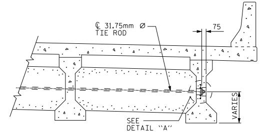
PART - SECTION AT INTERMEDIATE DIAPHRAGM
