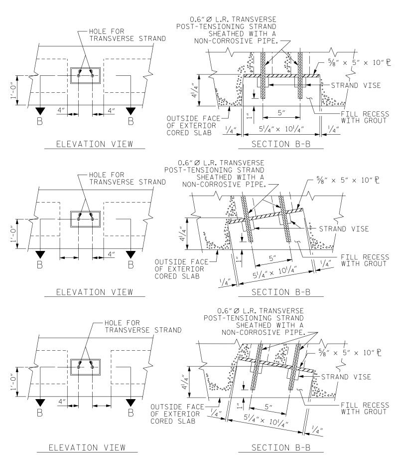
GROUTED RECESS AT END OF DOUBLE POST-TENSIONED STRANDS FOR CORED SLABS
