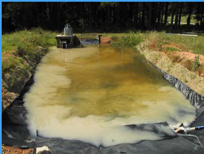
A model settling basin was used in the recently completed research on the use of polyacrylamide and baffles to reduce turbidity and TSS.
