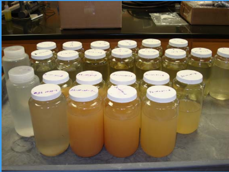
Flow-weighted samples of roadway runoff show the variation in turbidity that can be experienced under varying conditions and at different periods of the storm event.
