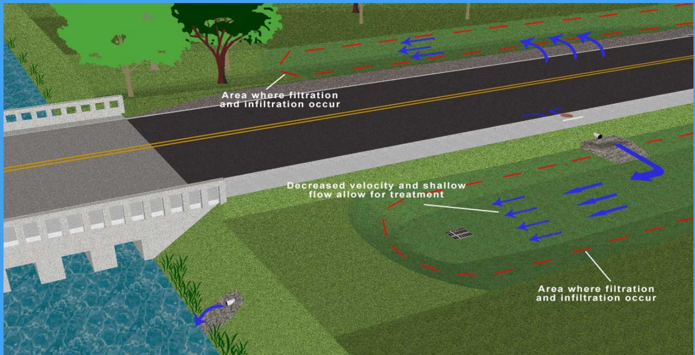
Schematic of a vegetated swale showing how it functions.
