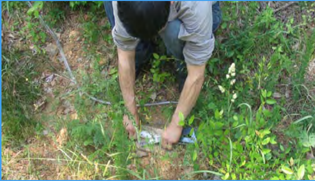
Researcher from UNCC placing a flow meter at a swale outlet in the Jordan Lake Watershed
