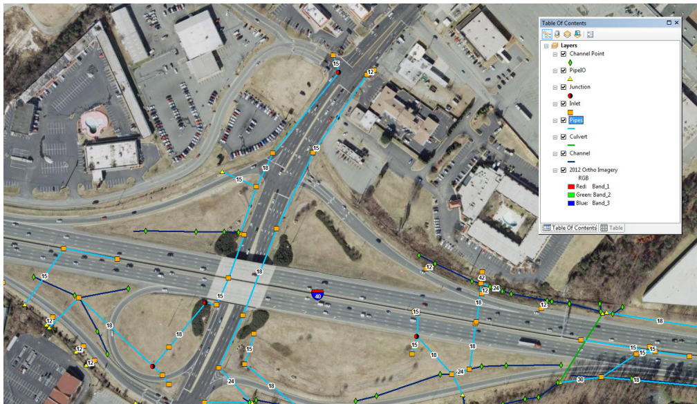
Resulting data collection showing drainage system connectivity
