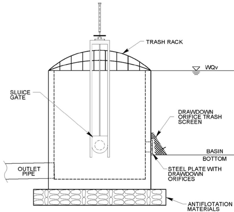
Figure 2-4. Outlet control structure
