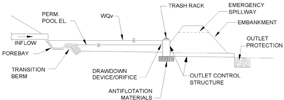
**Figure 12-3.** Profile view: wet detention basin cross section
