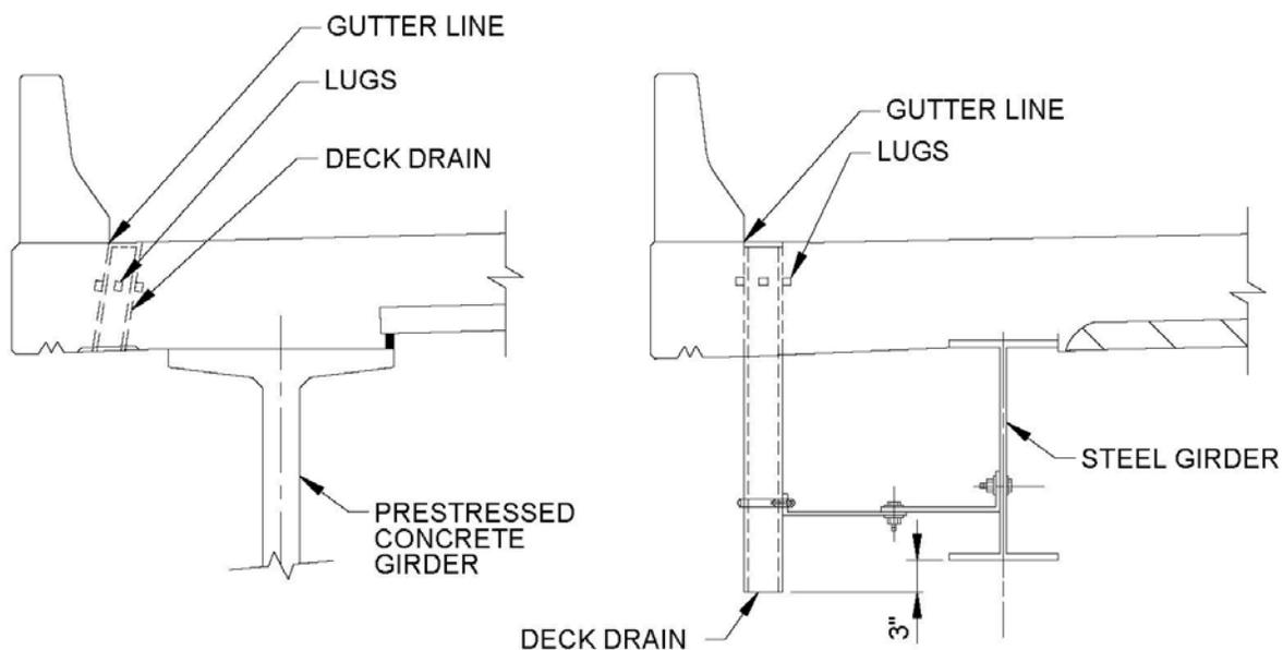
**Figure 9-5.** Deck drain orientation for prestressed concrete (left) and steel (right) girder bridges
