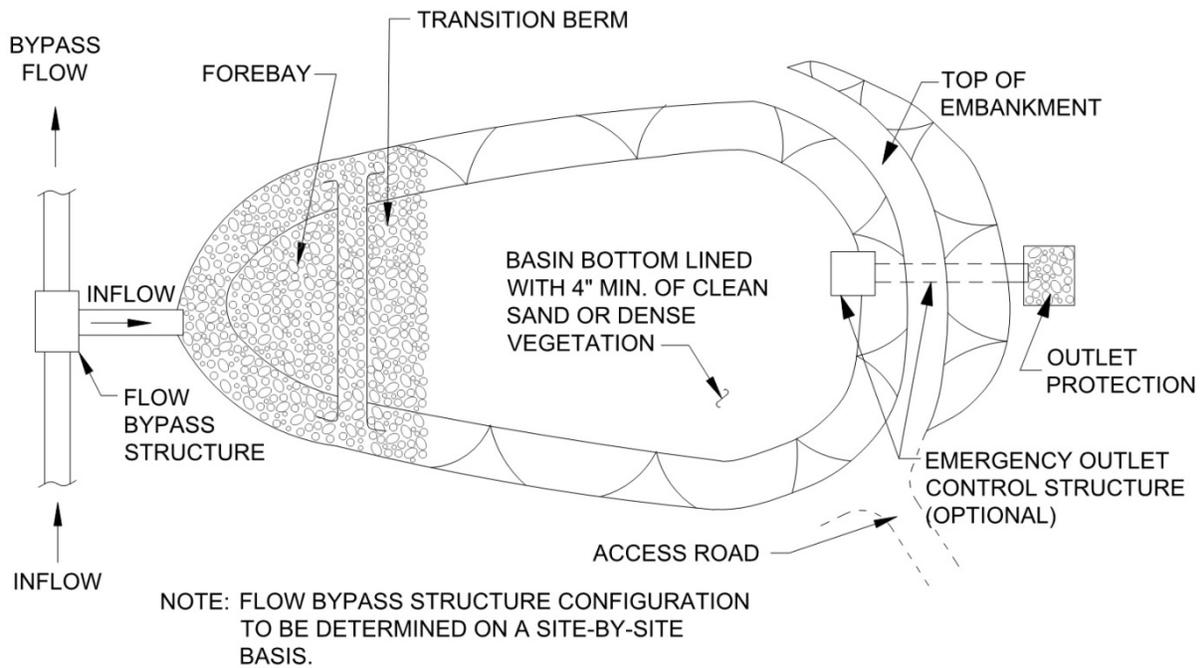
**Figure 10-1.** Plan view: infiltration basin and its components
