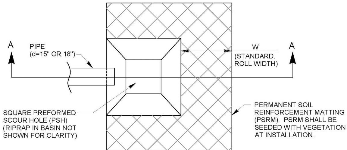
Figure 4-2. Plan view: typical preformed scour hole layout and components
