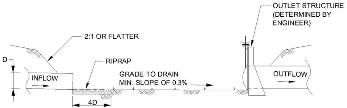
Figure 8-3. Profile view: hazardous spill basin cross section
