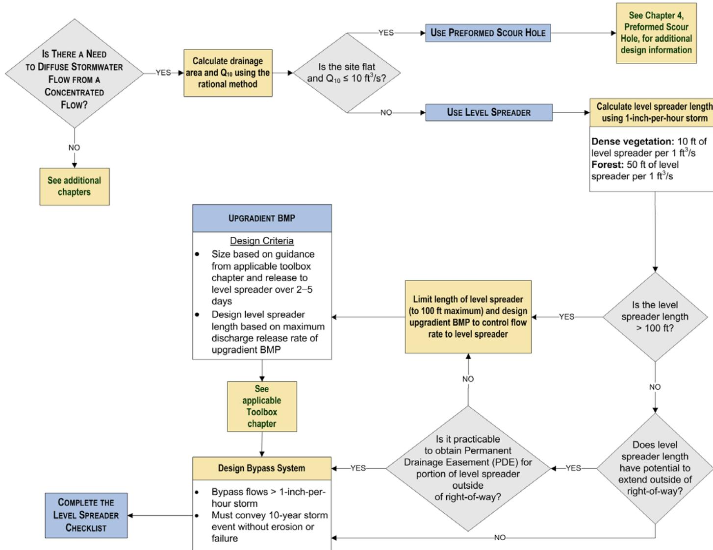
Figure 3-6. Level spreader design flowchart
