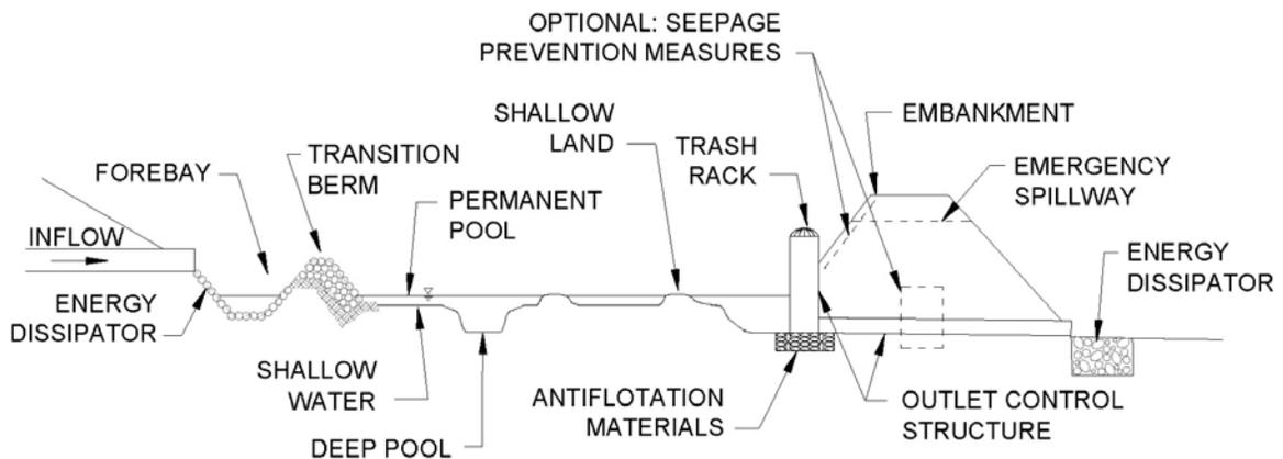
**Figure 13-3.** Plan view: stormwater wetland cross section
