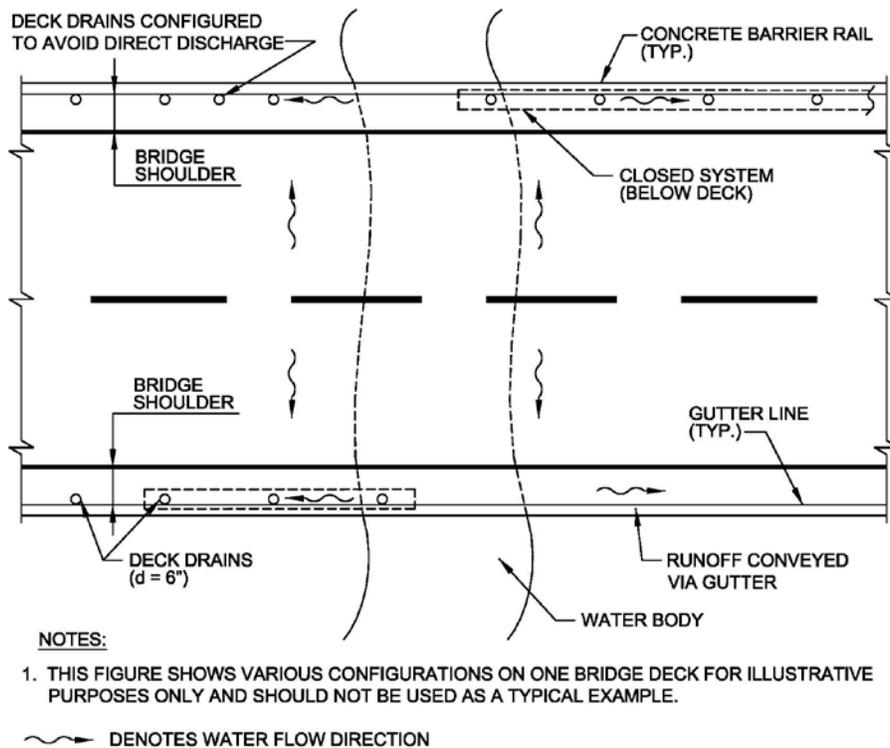
Figure 9-3. Plan view: varying bridge drainage conveyance configurations for a girder bridge
