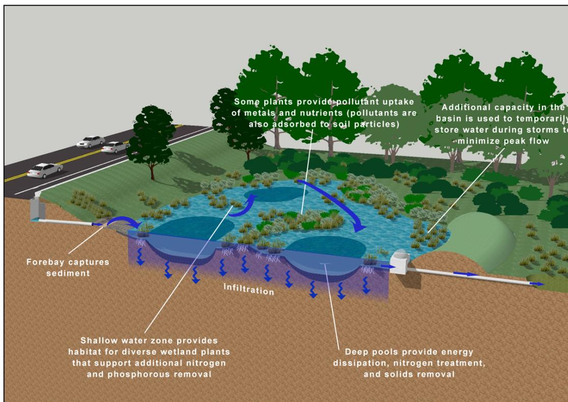
**Figure 13-4.** Typical stormwater wetland configuration and pollutant removal processes
