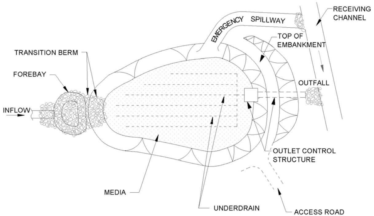
**Figure 11-1.** Plan view: media filter and its components
