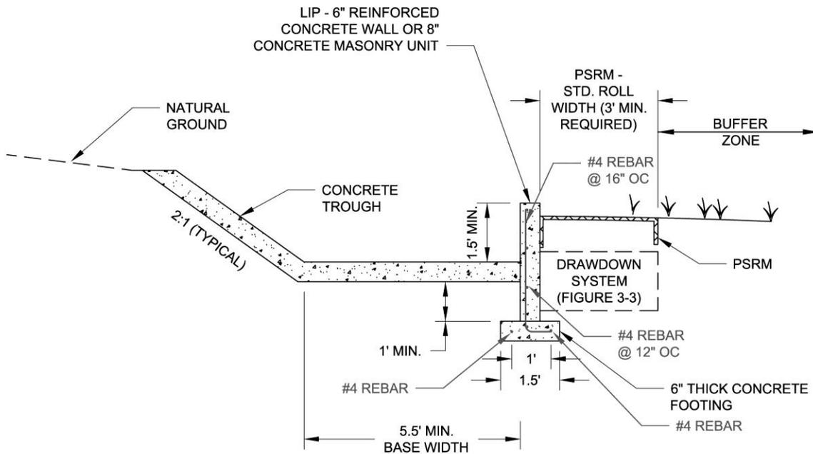
Figure 3-2. Profile View: typical level spreader details and components
