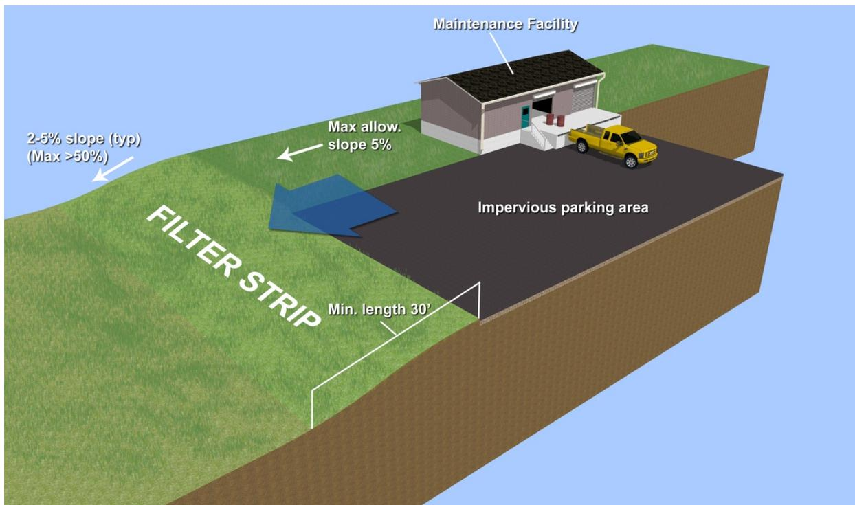
**Figure 14-3.** Typical non-road filter strip design components
