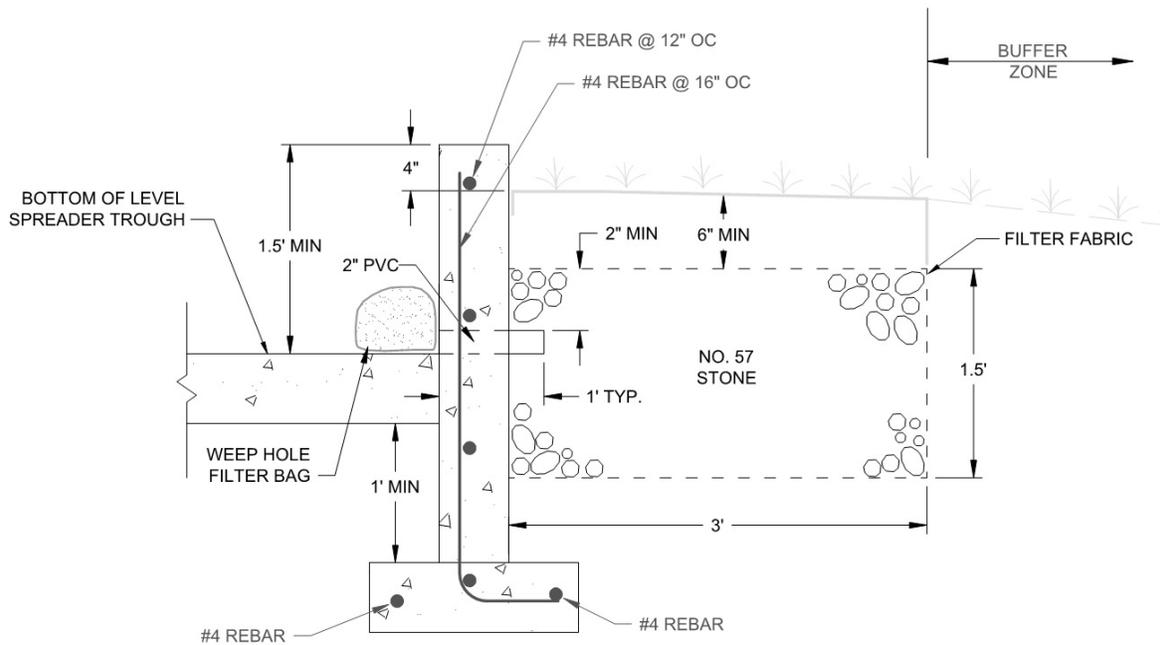
Figure 3-3. Profile view: weep hole dry cell detail for level spreader
