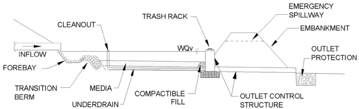
**Figure 11-2.** Profile view: media filter and its components
