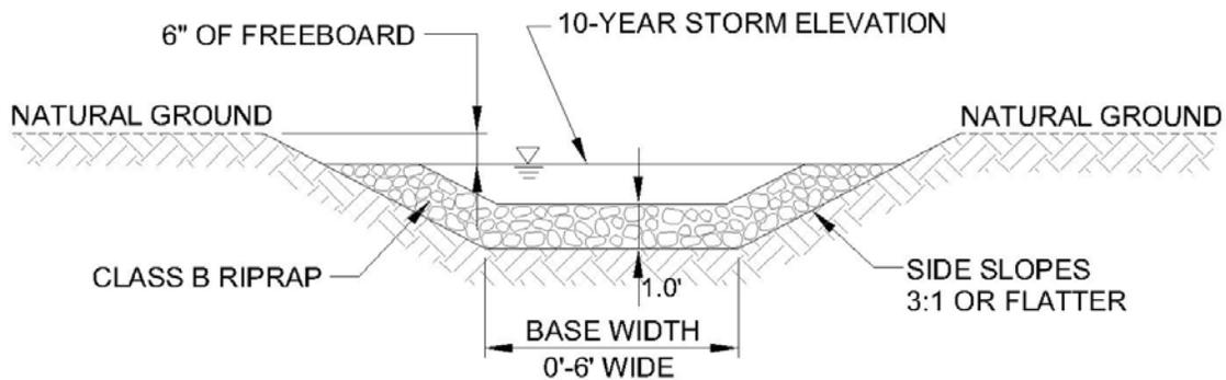
**Figure 6-3.** Profile view: swale cross section with optional water quality rock check
