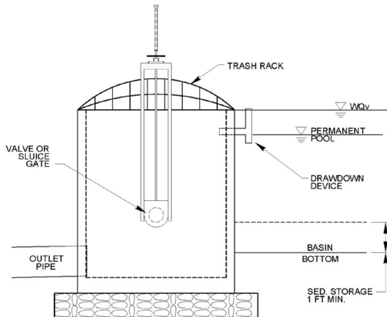
**Figure 12-6.** Wet detention basin outlet control structure
