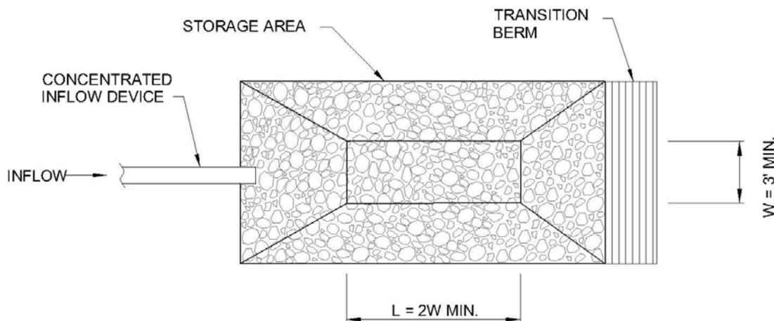
**Figure 7-2.** Plan view: typical riprap forebay layout and components
