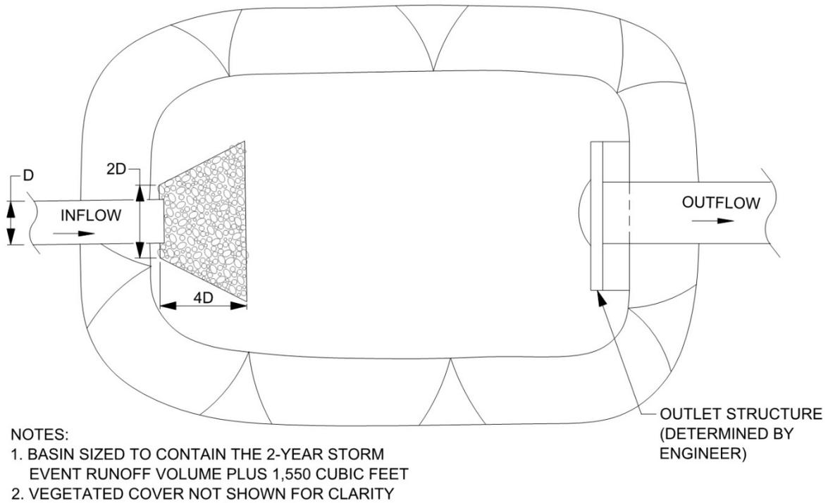
Figure 8-2. Plan view: typical hazardous spill basin layout and components
