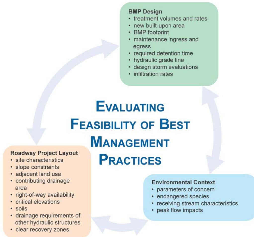
**Figure 2-2.** Common considerations for determining BMP feasibility and selection
