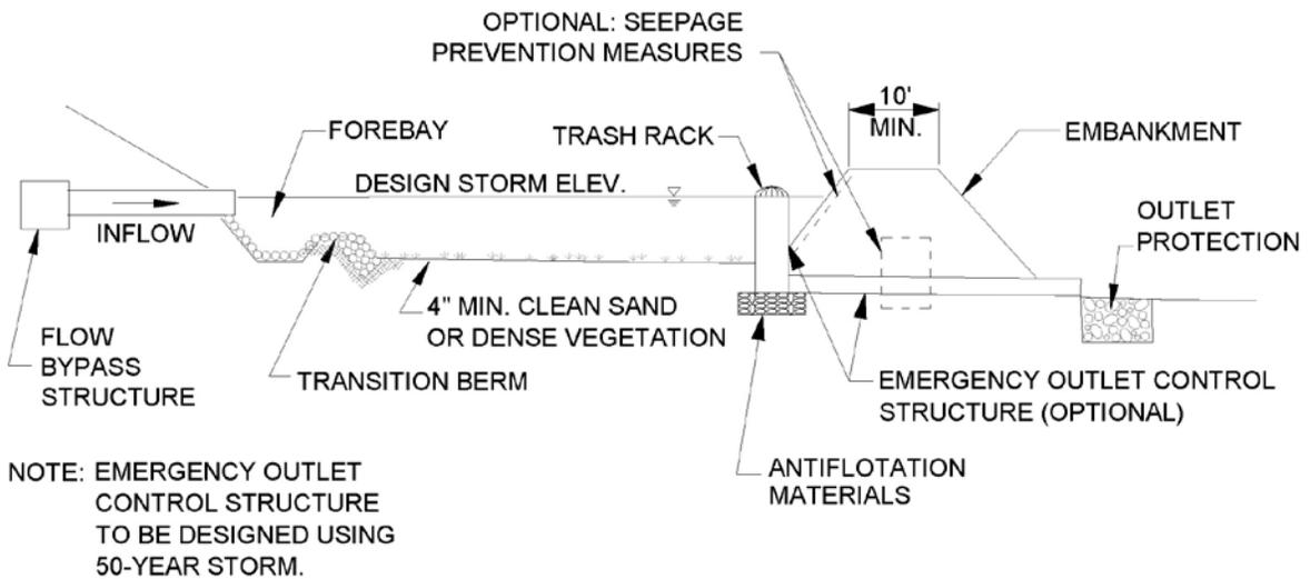
**Figure 10-2.** Profile view: infiltration basin and its components
