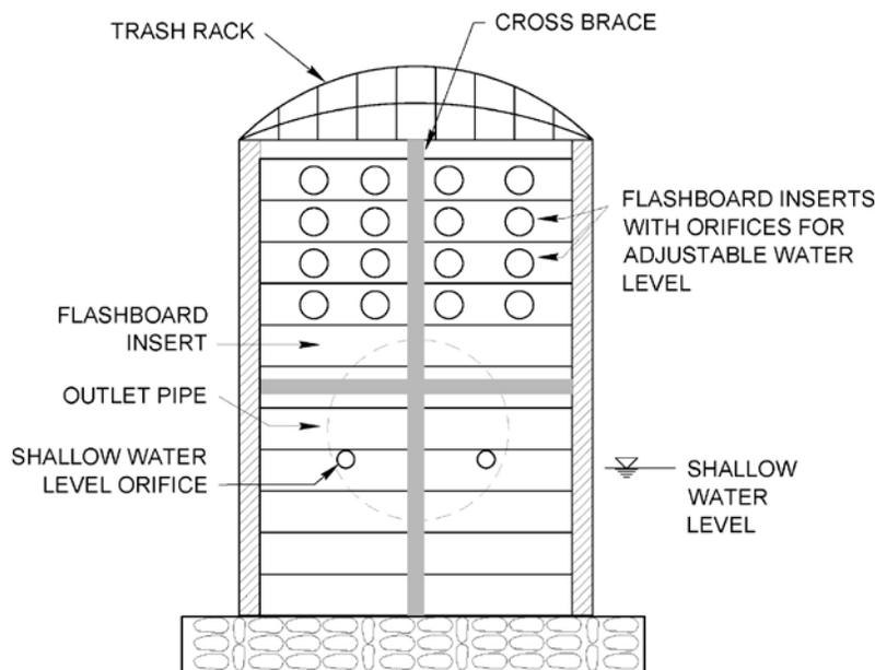
**Figure 13-5.** Typical flashboard riser outlet control structure
