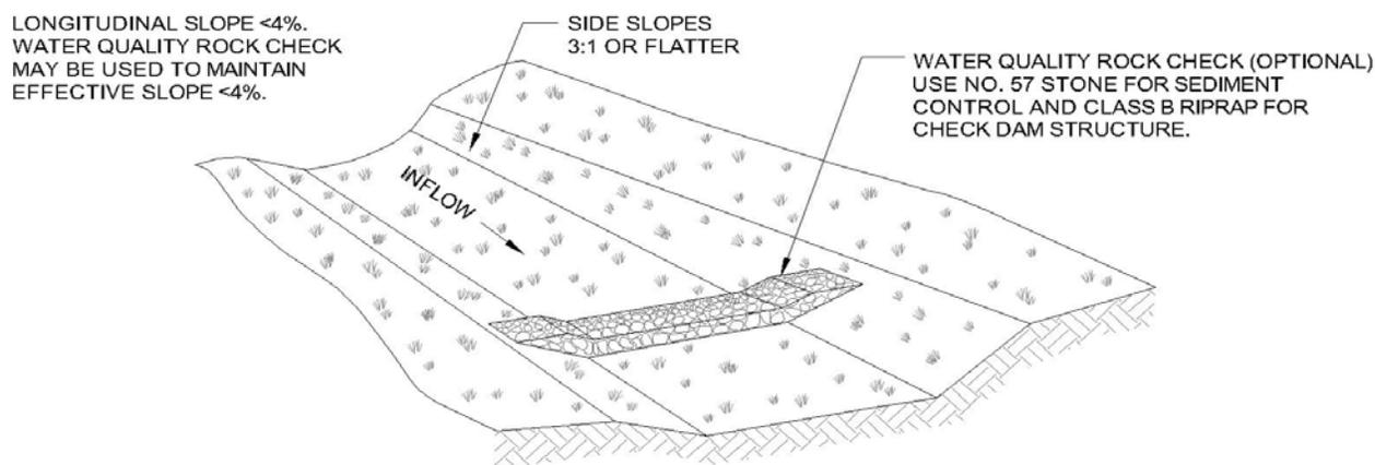
**Figure 6-2.** Isometric view: swale with optional water quality rock check
