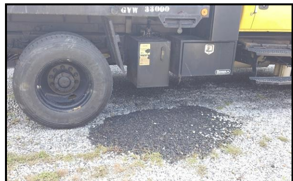
Hydraulic oil leak from NCDOT truck
