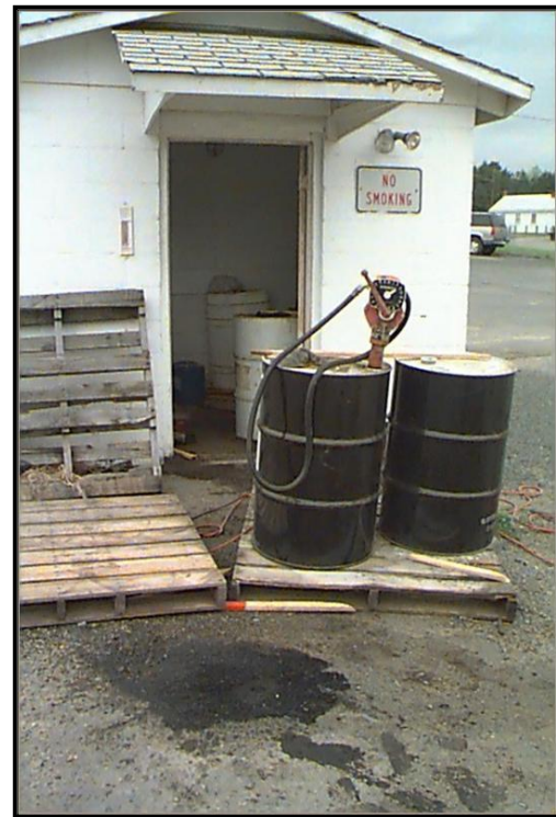
Stained pavement from spills outside drum storage/dispensing area
