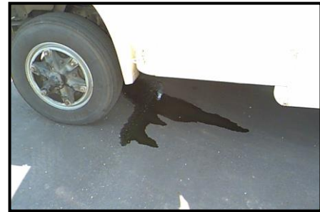
Antifreeze leak on pavement from NCDOT truck
