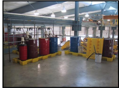
Drums of oil and hazardous substances stored on secondary containment pallets inside an NCDOT Equipment Shop
