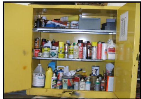
NCDOT self-contained flammables cabinet used to store HAZMATs
