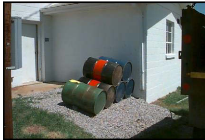
Empty drums stored horizontally on ground [Note: No cover or signage is provided]
