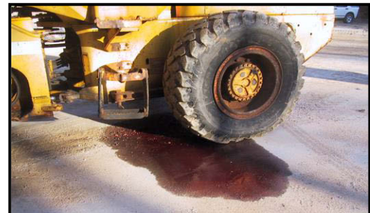
Hydraulic fluid spill on pavement from heavy equipment
