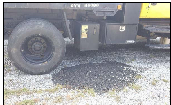
Hydraulic oil leak from NCDOT truck
