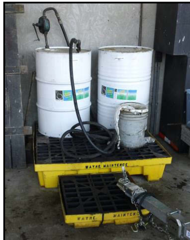
Asphalt release agent drums used to clean equipment [Note: excess cleaning product should be revised or properly disposed]
