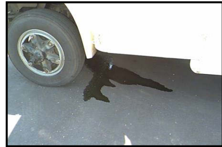
Antifreeze leak on pavement from NCDOT truck
