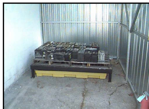
NCDOT batteries stored under cover on secondary containment pallet
