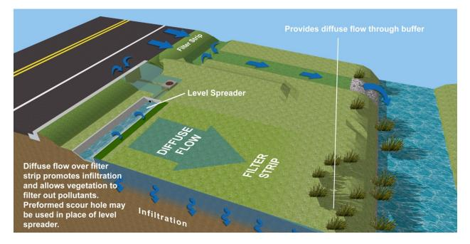
Figure 14-2. Typical filter strip configurations and pollutant removal processes
