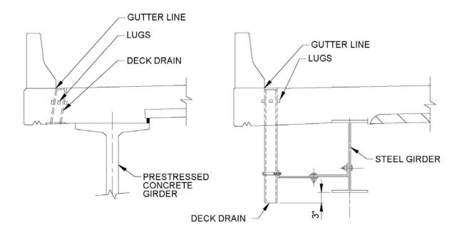
Figure 9-5. Deck drain orientation for prestressed concrete (left) and steel (right) girder bridges
