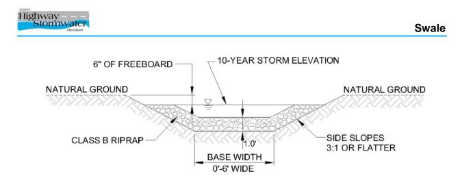
Figure 6-3. Profile view: swale cross section with optional water quality rock check
