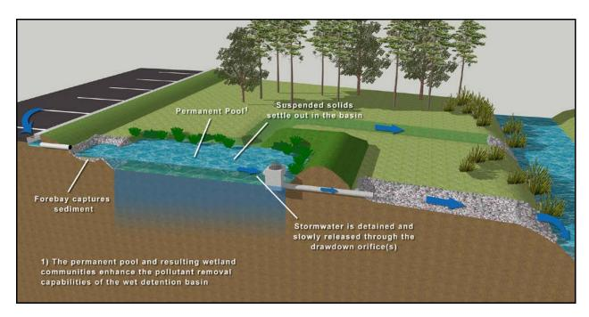
Figure 12-4. Typical wet detention basin configuration and pollutant removal processes
