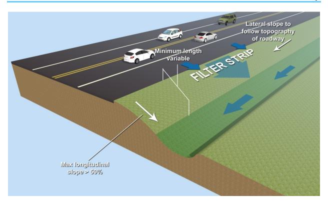
Figure 14-4. Typical roadway filter strip design components
