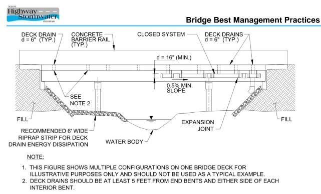
Figure 9-4. Profile view: varying bridge drainage conveyance configurations for a girder bridge
