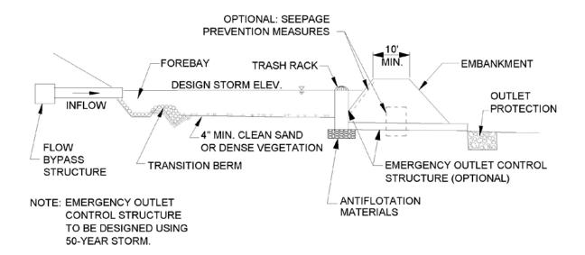
Figure 10-2. Profile view: infiltration basin and its components
