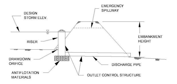
Figure 2-5. Detention basin components
