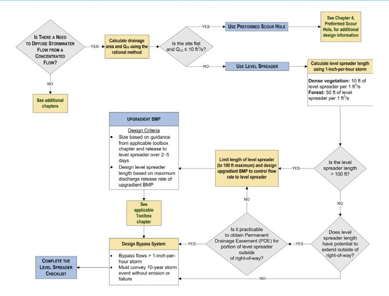
Figure 3-6. Level spreader design flowchart
