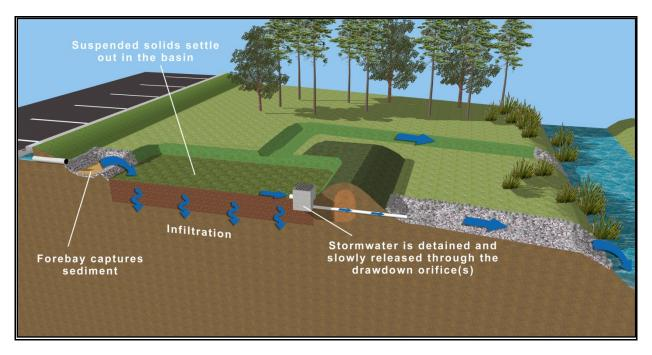
Figure 5-4. Typical dry detention basin configuration and pollutant removal processes
