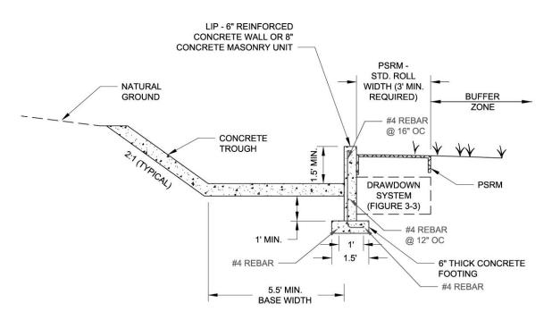
Figure 3-2. Profile View: typical level spreader details and components
