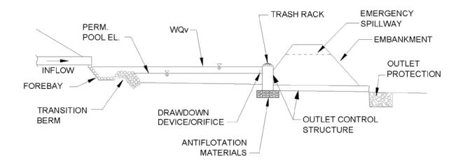
Figure 12-3. Profile view: wet detention basin cross section
