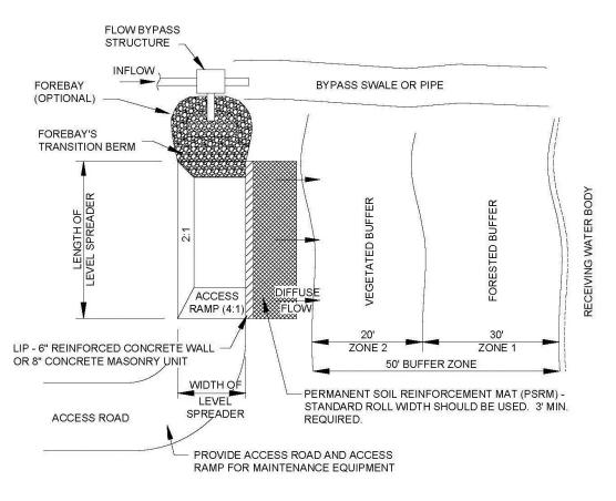
Figure 3-1. Plan view: typical level spreader layout with buffer
