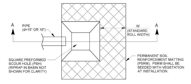
Figure 4-2. Plan view: typical preformed scour hole layout and components
