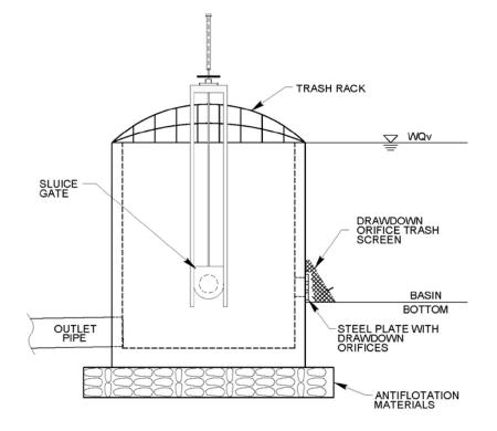
Figure 2-4. Outlet control structure
