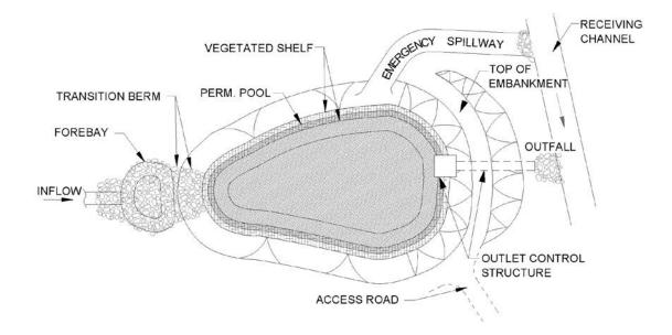
Figure 12-2. Plan view: typical wet detention basin layout and components
