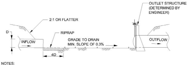
DURING NORMAL OPERATION, OUTLET STRUCTURE DOES NOT OBSTRUCT FREE FLOW OF RUNOFF
