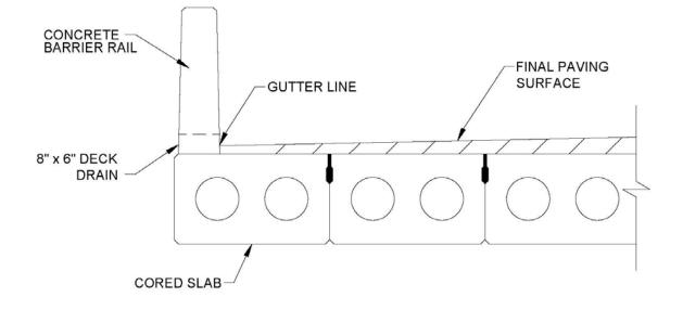
Figure 9-6. Deck drain orientation for cored slab bridges
