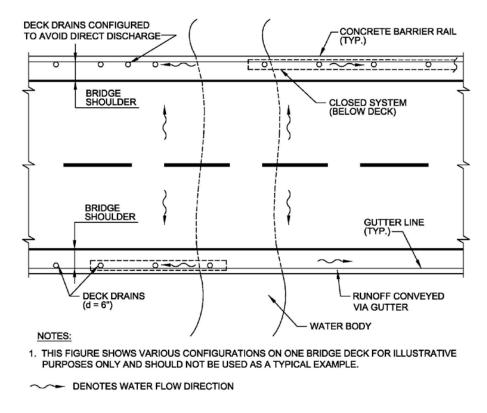
Figures 9-3 and 9-4 show various bridge drainage conveyance components and configurations.
