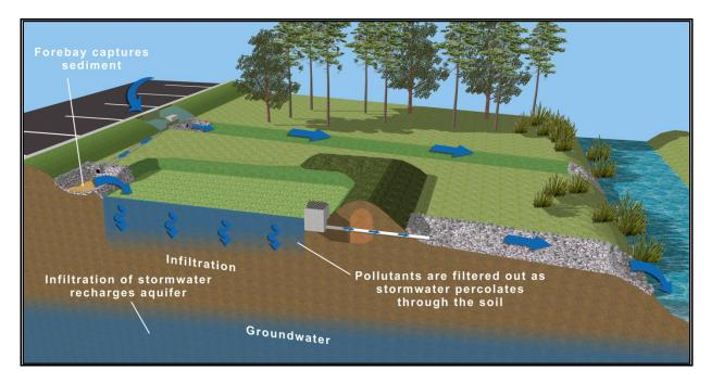
Figure 10-3. Typical infiltration basin configuration and pollutant removal processes
