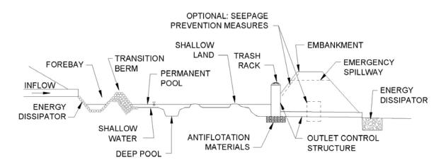
Figure 13-3. Plan view: stormwater wetland cross section
