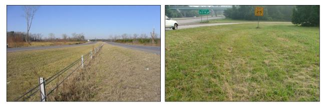
Figure 6-4. Linear highway applications of swales
