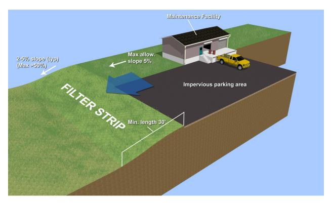
Figure 14-3. Typical non-road filter strip design components
