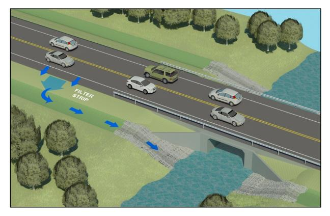
Figure 14-5. Example of conveyance designed downstream of filter strip to protect buffer and streambank from erosion
