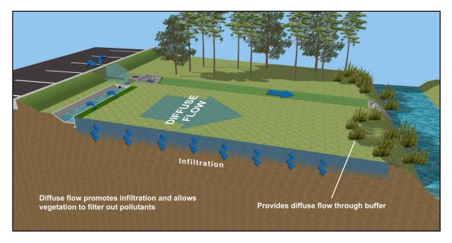
Figure 3-5. Typical level spreader configuration and pollutant removal processes
