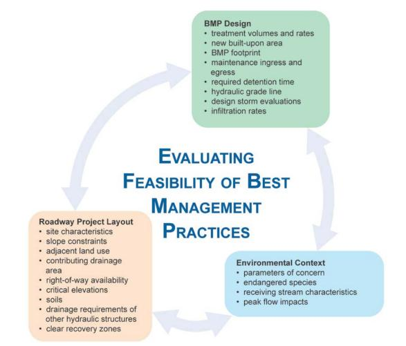
Figure 2-2. Common considerations for determining BMP feasibility and selection
