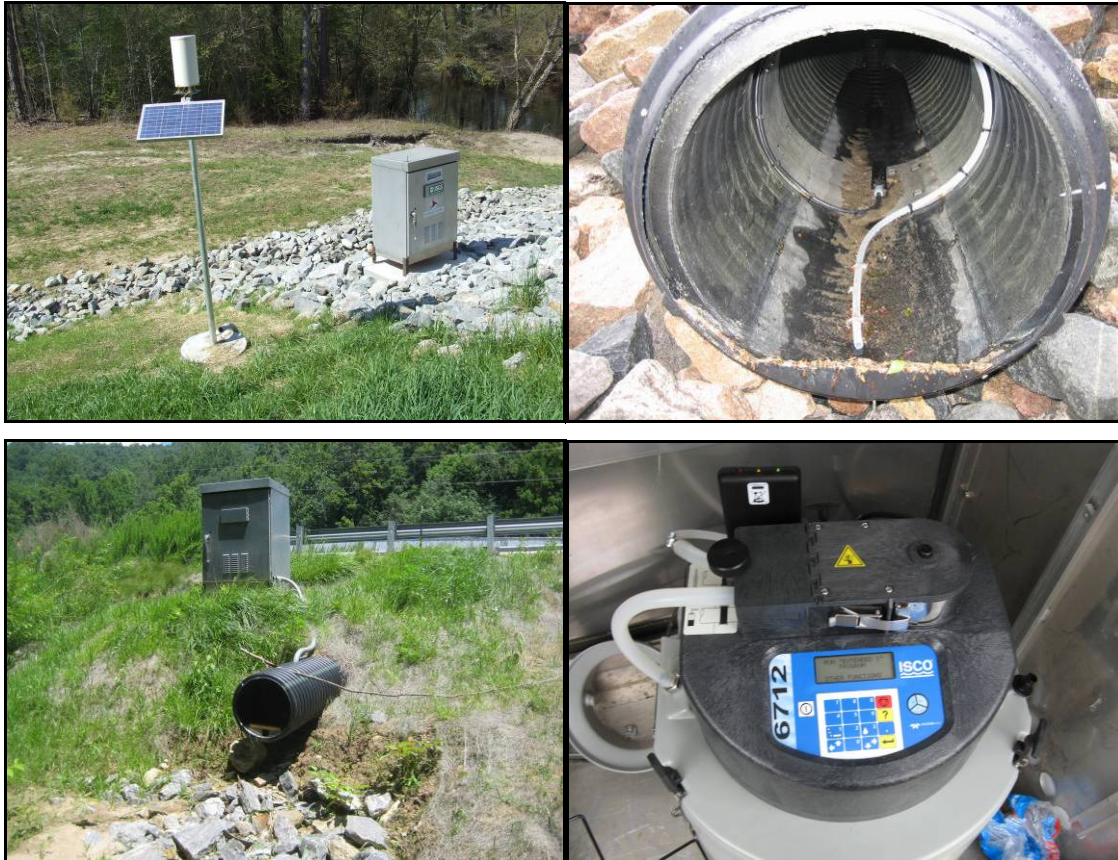
Figure 3.2-3: USGS bridge deck runoff monitoring equipment: (clockwise from top left) tipping bucket rain gage and autosampler monitoring box; autosampler intake tube, diffuser plate, velocity meter and pressure sensor inside discharge pipe; ISCO autosampler inside monitoring box; and monitoring box with autosampler intake tube and conduit connection to pipe outlet.
