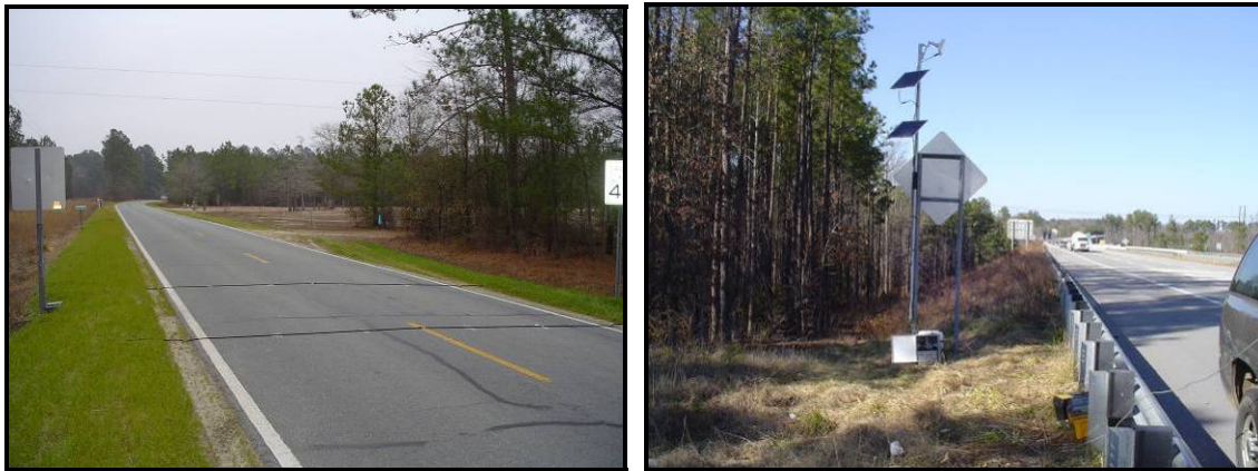
Figure 3.5-1: Traffic survey devices. Pneumatic road tubes installed on NC 411 near Bridge No. 810014 over Black River (left photo) and radar device installed on shoulder of I-540 near Bridge No. 911102 over Mango Creek (right photo).
