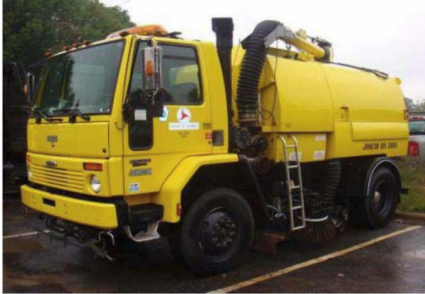
Figure 3.3-4: Bridge sweeping equipment: Allianz Johnston VT650 sweeper.
