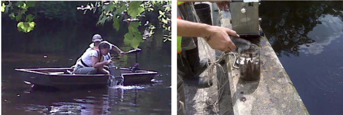
Figure 3.3-2: Instream (left) and bridge deck (right) streambed sediment sampling.
