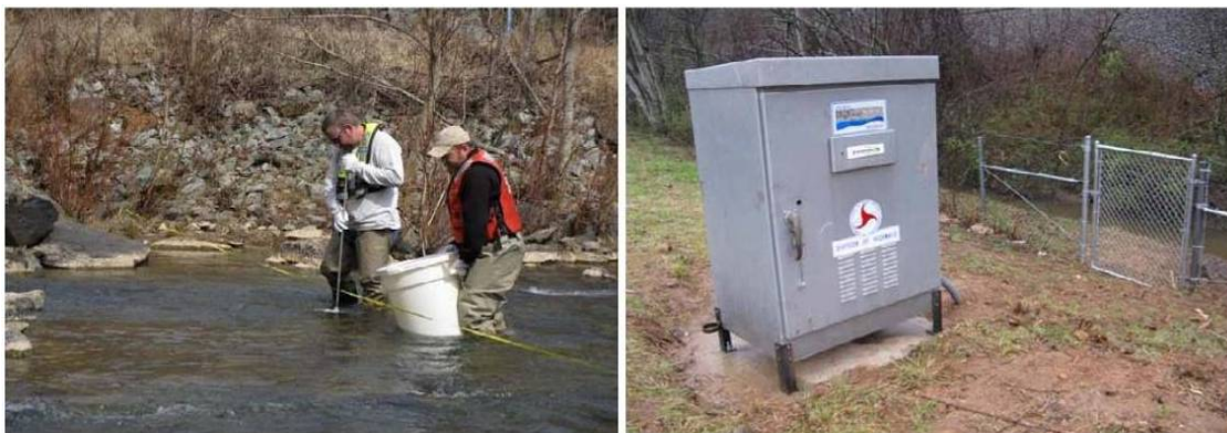
Figure 3.2-5: Instream sampling methods and techniques: EWI method (left) and automated samplers inside monitoring box (right).
