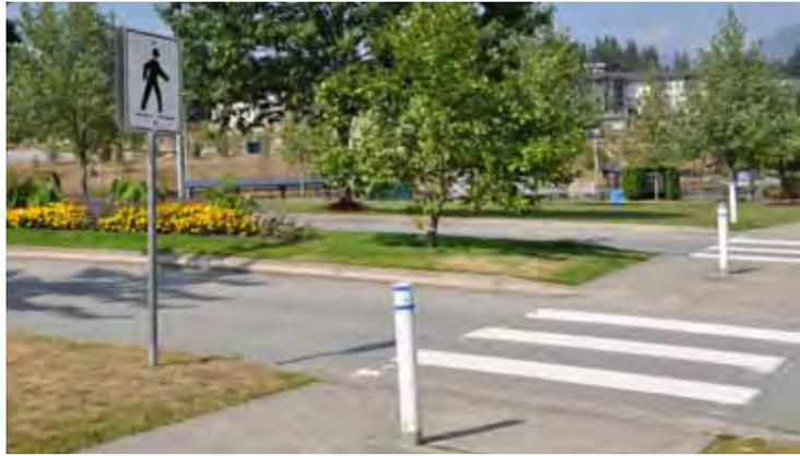
This crosswalk includes stripes in the roadway, bollards to protect pedestrians, and signage to delineate the walks. Image courtesy DepositPhotos.com.
