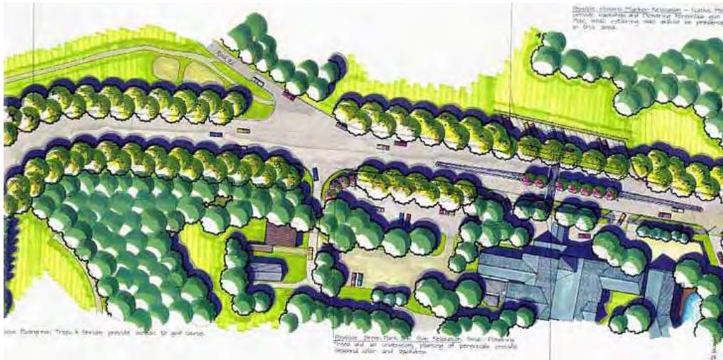
A conceptual plan for US 321 near Blowing Rock, North Carolina, shows how mass plantings would help define the corridor. Image courtesy NCDOT.
