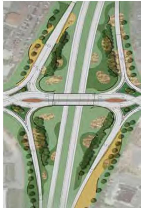
*This diagram of the diverging diamond interchange on I-77 in North Carolina shows the way landscaping helps enhance the intersection by softening the visual impact of the access ramps. Image courtesy NCDOT.*
