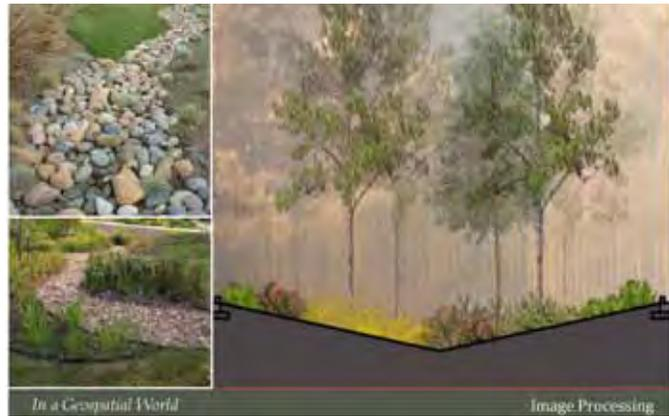
The Texas Land and Water Forum conducted a Low Impact Development (LID) competition in 2009 to explore how LID could be implemented in Harris County. The winning entry for Independence Parkway pushed the roadways to the edge of the right-of-way and created a bioswale in the median. This bioswale is able to handle all run-off from a 100-year storm and it also reduces sedimentation and pollution runoff, and significantly improves aesthetics. Image courtesy AECOM.
