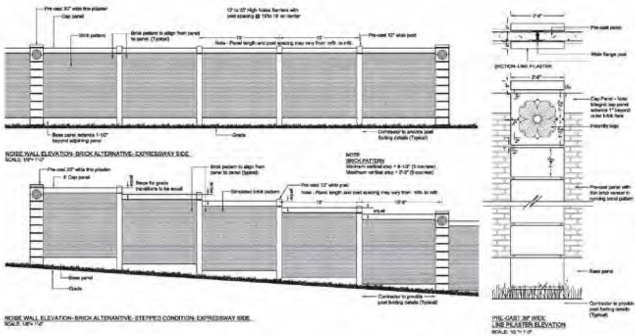
These elevations show the level of detail to be implemented as part the the noise walls used for the Triangle Expressway in Raleigh, North Carolina. The top elevation shows a noise well along level ground, while the bottom elevation shows how the walls would step down to follow the grade for steeper slopes. Image courtesy NCDOT.
