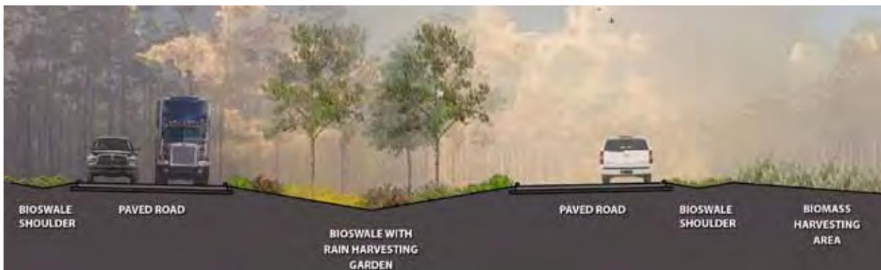
*Pushing the travel lanes out to the far edges of the right of way provide space for a wide bioswale for rain harvesting. This image is of Independence Parkway in Houston, Texas, and was prepared for the Texas Land and Water Forum's Low Impact Development Competition. Image courtesy AECOM.*
