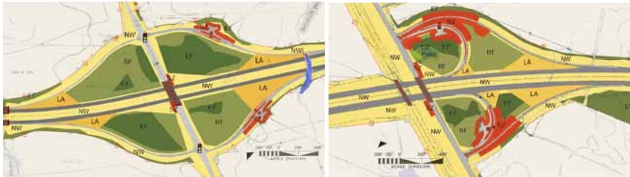
These plans outline the basic aesthetic guidelines for planting along various interchanges that are part of the Triangle Expressway. These plans provide a template that can be applied to all of the interchanges that are part of the project. Image courtesy NCDOT.
