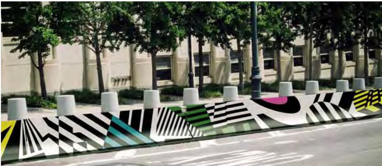
*The use of bold, angular geometric forms painted on jersey barriers helps blur the barrier's edges and soften the visual impact. This approach is intended to induce nearby traffic to slow down, producing a safer, more bike- and pedestrian-friendly thruway. Image courtesy John Locke.*
