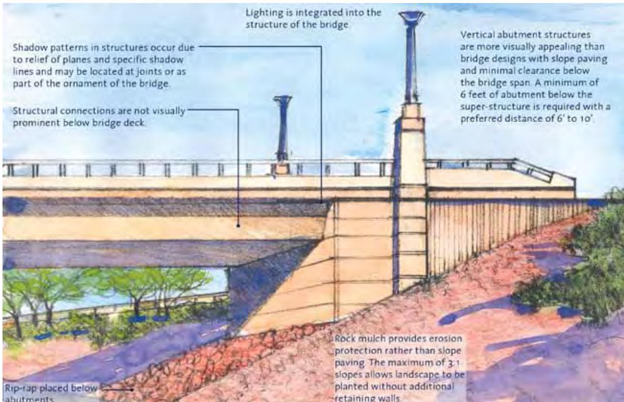
*This sketch shows concepts for how to integrate the railings, columns, bridge deck, abutment, and landscaping for a bridge over I-15 in Las Vegas, Nevada. The sketch shows the use of shadow patterns, integrated lighting, vertical abutments structures, rock mulch and rip-rap, and structural connections. Image courtesy NVDOT.*
