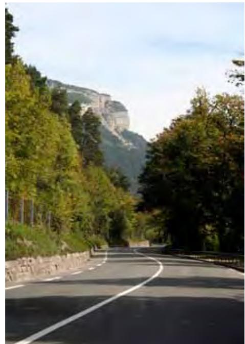
*The stone walls on the left and guardrail on the right allow trees to be close to the road in this photograph from western North Carolina. Image courtesy DepositPhotos.com.*
