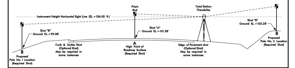
Step 2: Find the elevation difference between Shot "A" and Shot "B"
