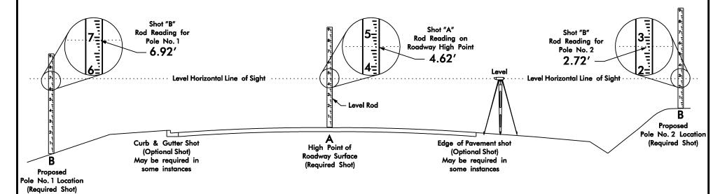
Step 2: Find the elevation difference between the proposed foundation and the high point of the roadway
