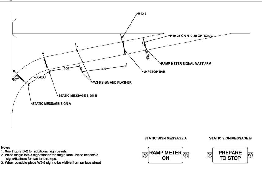
Figure E-3: Freeway-to-Freeway Ramp Meter Signing and Pavement Markings
