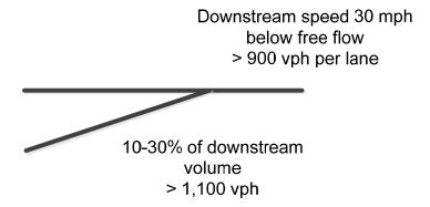
Figure 1: Typical Criteria for Ramp Metering
