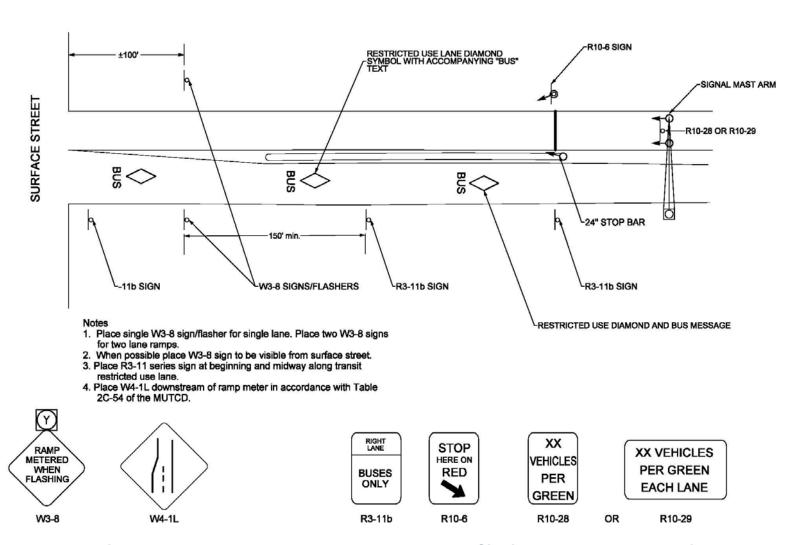
Figure E-1: Non-Freeway-to-Freeway Ramp Meter Signing and Pavement Markings
