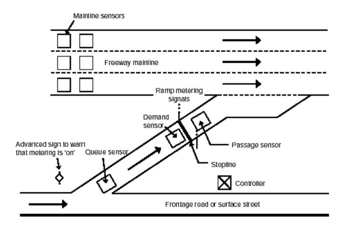
Figure 3: Typical Ramp Meter Site Layout
