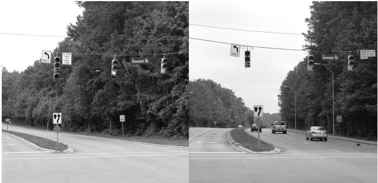
1 FIGURE 1 Photographs of FYA-PPLT (Left) and FYA-Permissive Only (Right) left turn displays
