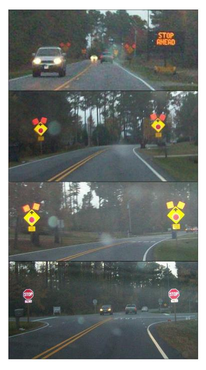
Figure 3 Signing and Marking on a Recently Converted 45-mph Approach
