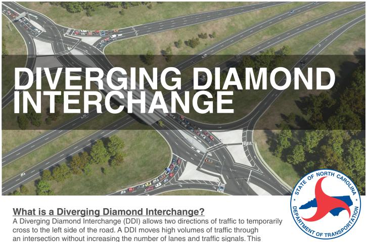
cross to the left side of the road. A DDI moves high volumes of traffic through an intersection without increasing the number of lanes and traffic signals. This movement provides easier access to an interstate.
