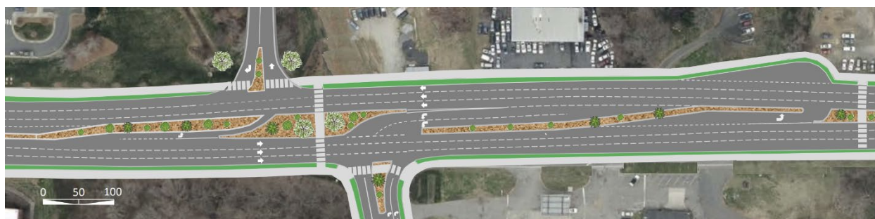
Figure 15. Offset RCI concept to provide 90-degree crosswalk.
