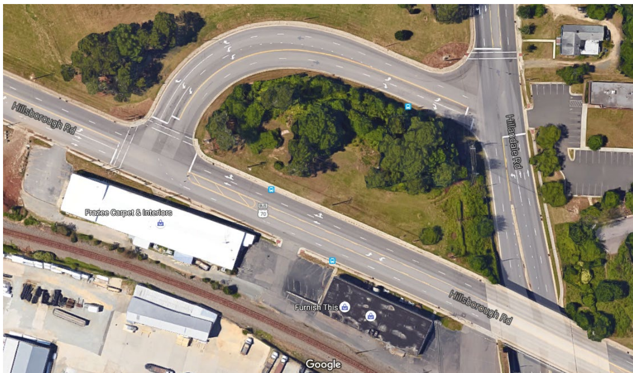
Figure 26. Example grade-separated intersection using a connector road (Hillsborough Road at Hillandale Road in Durham).
